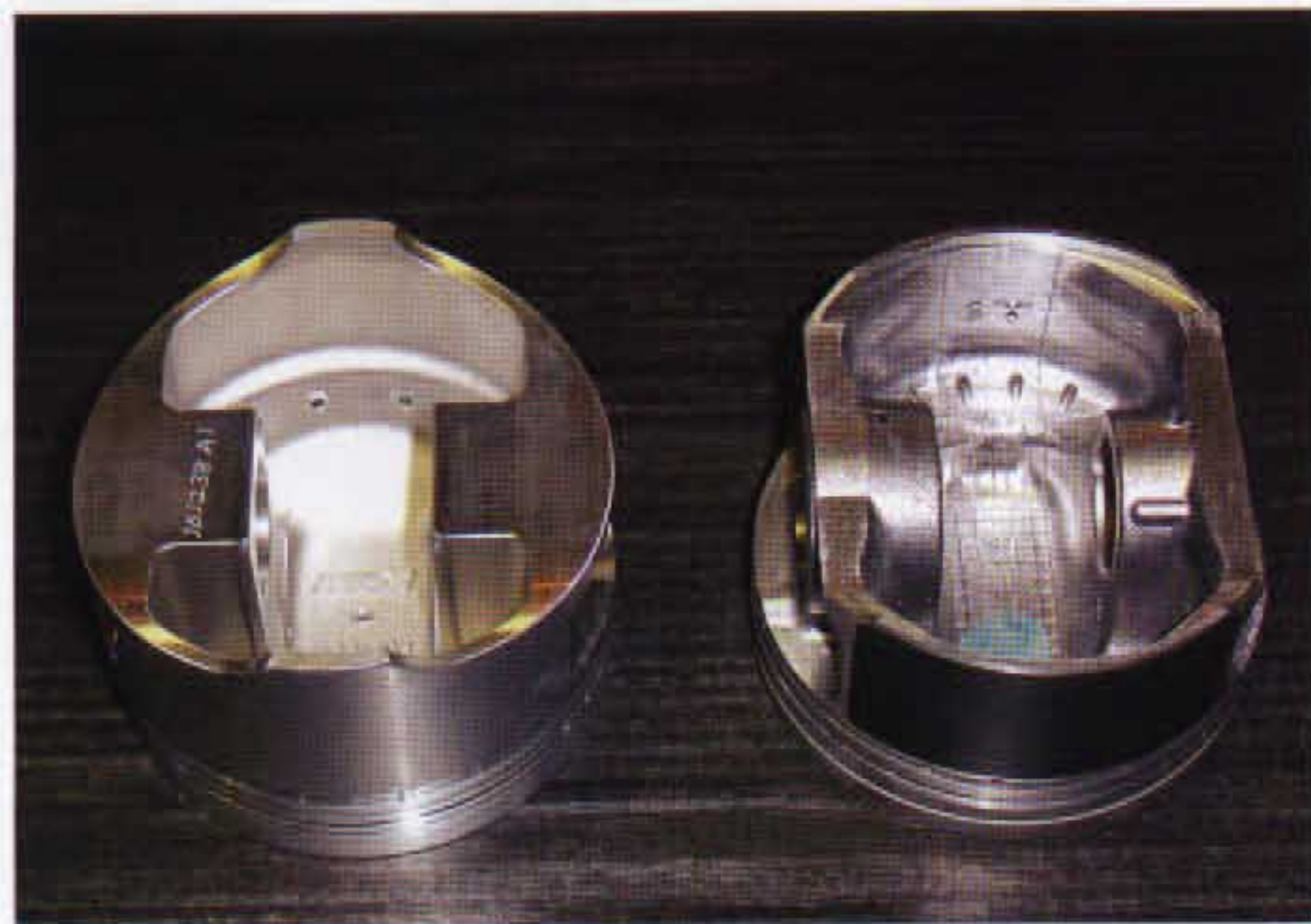
Ross 8.8:1 piston on left versus stock piston on the right.
