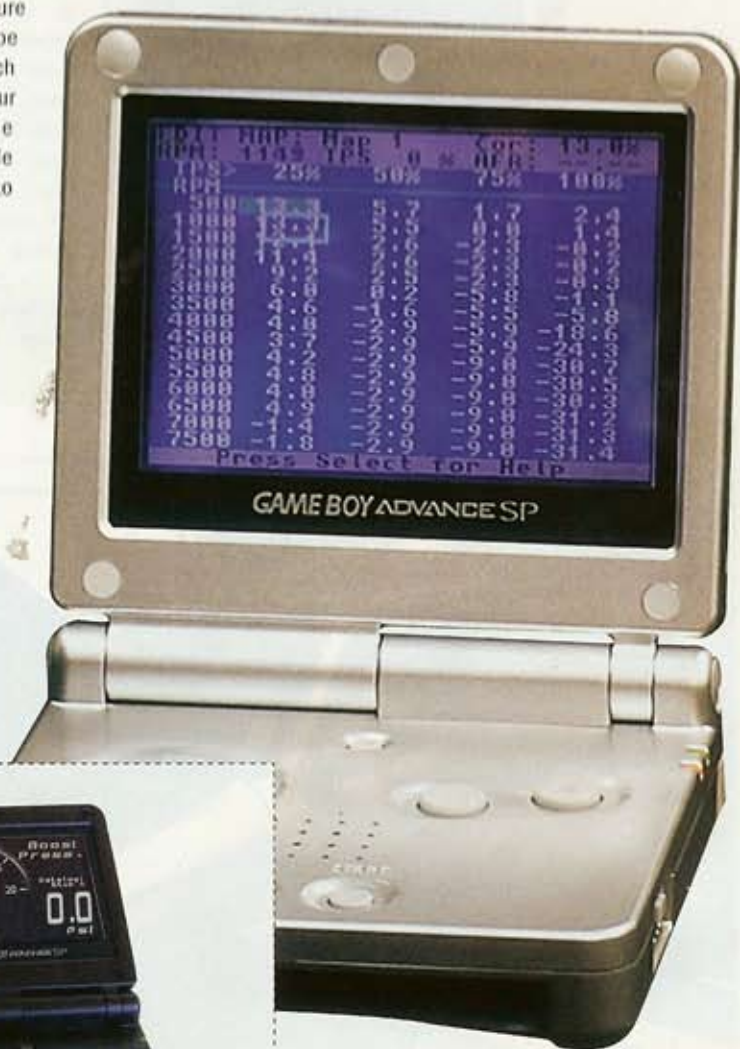
Shown here is a typical DTEC map layout. From here you can add or subtract values.
