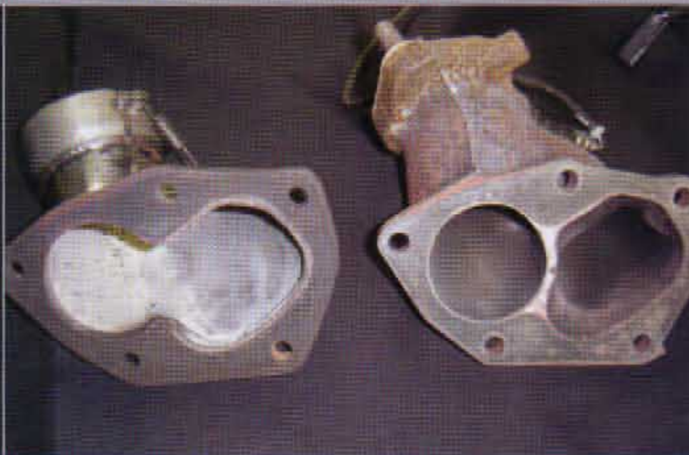
AMS hogged out O2 housing vs Stock EVO housing
