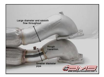
Unlike the copy, the AMS EVO X Widemouth Downpipe provides optimal flow throughout without the rough transition into a smaller diameter pipe. If the rough transition on the copy is not apparent, the image on the following page will surely illustrate that it is.
