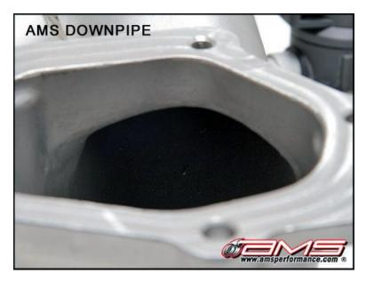
Seen above, the AMS downpipe offers completely smooth flow. There is no obstruction or a need to worry about premature corrosion. Our materials show no magnetic properties which indicate that it's made of cast 304 grade stainless steel. Our pipe was truly "designed to last the lifetime of your vehicle".
