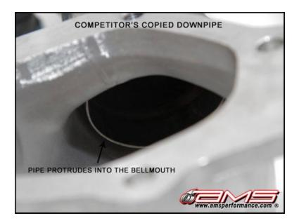
Here you can see the competition took an inferior approach. Rather than spending the extra cost to completely cast the bellmouth section, they decided to slip a pipe into the mouth and weld it to keep costs down. This was a bad choice as they added another weld which greatly compromises strength on a part that has to endure extreme heat/cooling cycles and stress.
