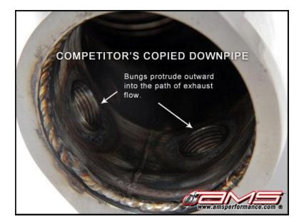
The  $O_2$  bungs also protrude into the path of exhaust flow creating additional turbulence and yet another area for corrosion to prematurely take effect. If you compare the image of our downpipe's lower section with the competitor's lower section, you will notice that ours is still cast and smooth throughout.
