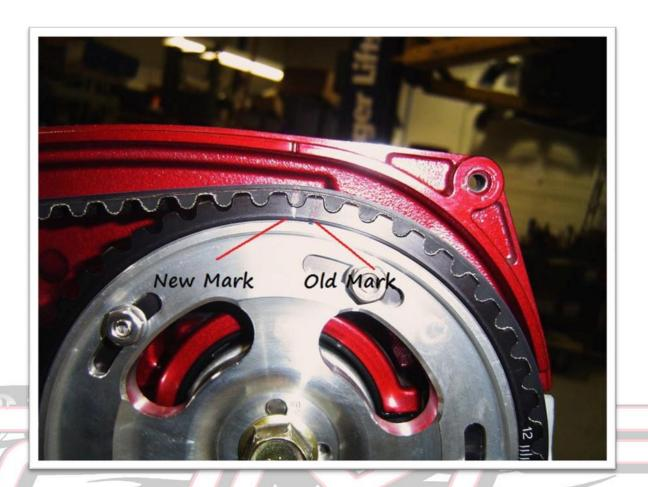
Because the cams are pulled slightly forward due to the custom deck height, you will need to retard the cams 3.75 degrees to get them to "factory" position.
