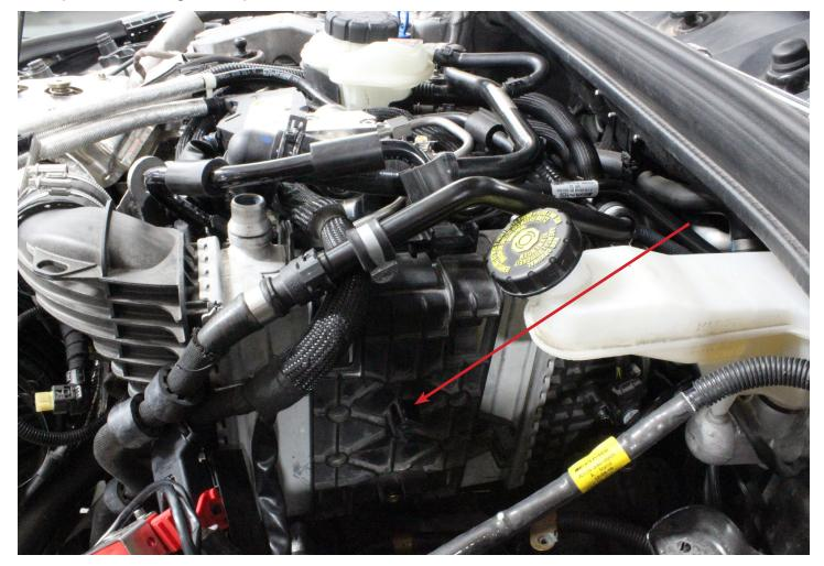
**13)** Remove the factory MAP sensor that is fastened to the OEM intercooler and install it onto the flange on the Alpha Intercooler using the supplied hardware. Make sure NOT to reuse the OEM bolts as damage will occur to the new intercooler.
