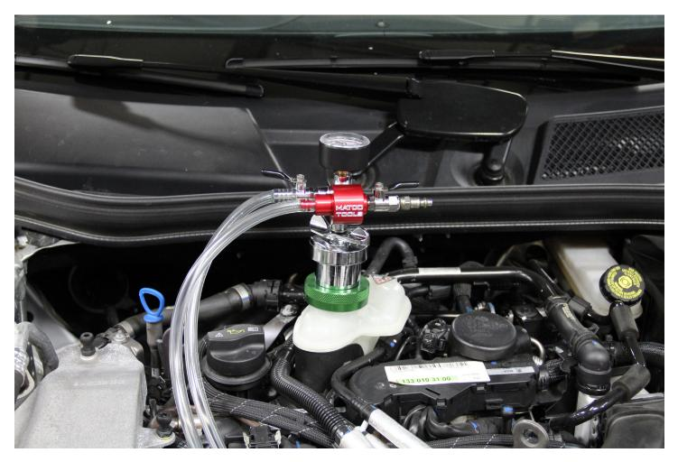
**3)** Use the air lift system to fill the system with coolant according to the tool's instructions. Once filled, remove the air lift tool.
