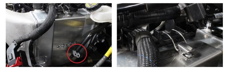
Note: Replace the OEM clamps on the compressor discharge and intercooler outlet coupler with the two #40 and one #56 clamp provided. Make sure to tighten the clamp as close to the bead on the inlet and outlet to deter movement.
