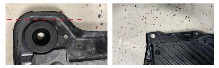
**17)** The air box mounting bracket may also need trimming. Test fit the air box and trim the mounting bracket as necessary to clear the intercooler end tank.
