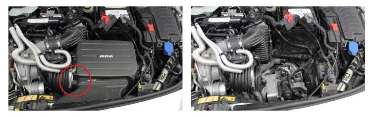
**6)** Drain the intercooler system. The lowest point in the system is the lower water hose connector on the side heat exchanger on the right side of the vehicle. Remove the fender liner and drain the system from there. The system can also be drained from the bottom connection on the intercooler or the intercooler pump however it will be a little messier.
