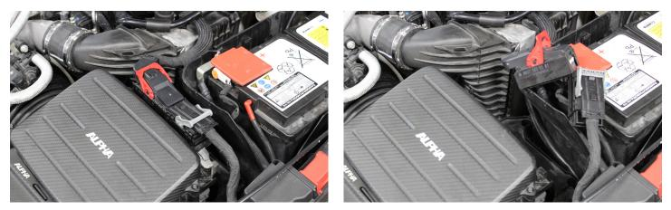
**4)** Disconnect the MAP sensor on the air box. To do so, use a small screwdriver to pull out the grey tab from the connector. Once released, depress the grey tab down to disconnect.
