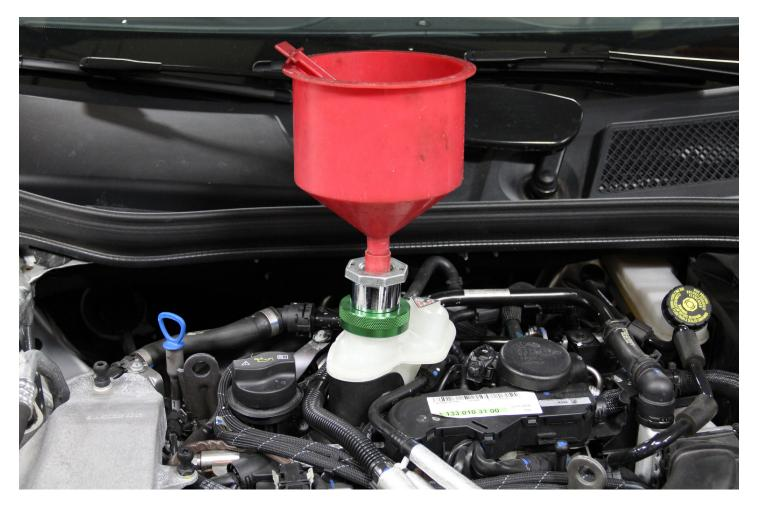
**2)** It may only take a little bit of coolant. Close the bleeder and run the car until the IC pump turns on. This can take 10 minutes or more of idle time.
