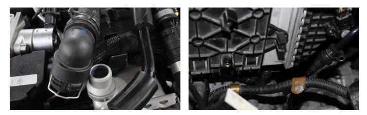
**10)** Disconnect the small quick connect line going into the top of the intercooler outlet end tank as well as the MAP sensor harness on the side.
