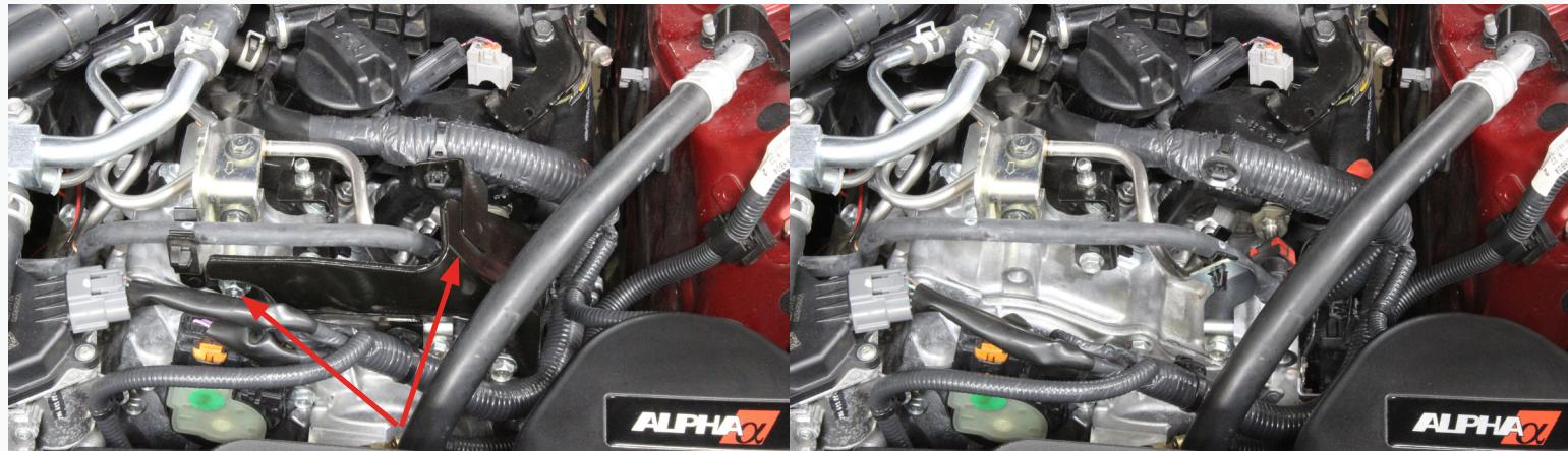
3) If equipped, remove the 10mm bolt and bracket bolted to the intercooler holding the sound deadening cover for the HPFP. Disconnect the connector at the HPFP and remove the cover.
