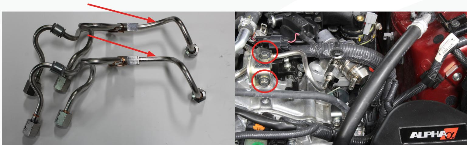
12) On the STAGE 3 HPFP, we have supplied a high pressure line template. The template is 3D printed and aids in the bending of the line properly. This tool is not used to bend the line but to check it being bent correctly. The plastic template slides over
