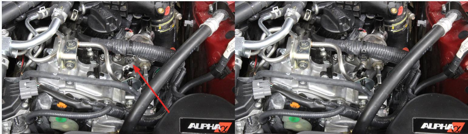
6) Loosen but do not remove the two 10mm bolts on the bracket supporting the high pressure line. Unbolt the HPFP but do so in steps loosening the bolts one turn at a time. You must do this due to the possibility of cam shaft lobe being at the top and the HPFP being under the load from its return spring. Remove the HPFP once fully disconnected.
