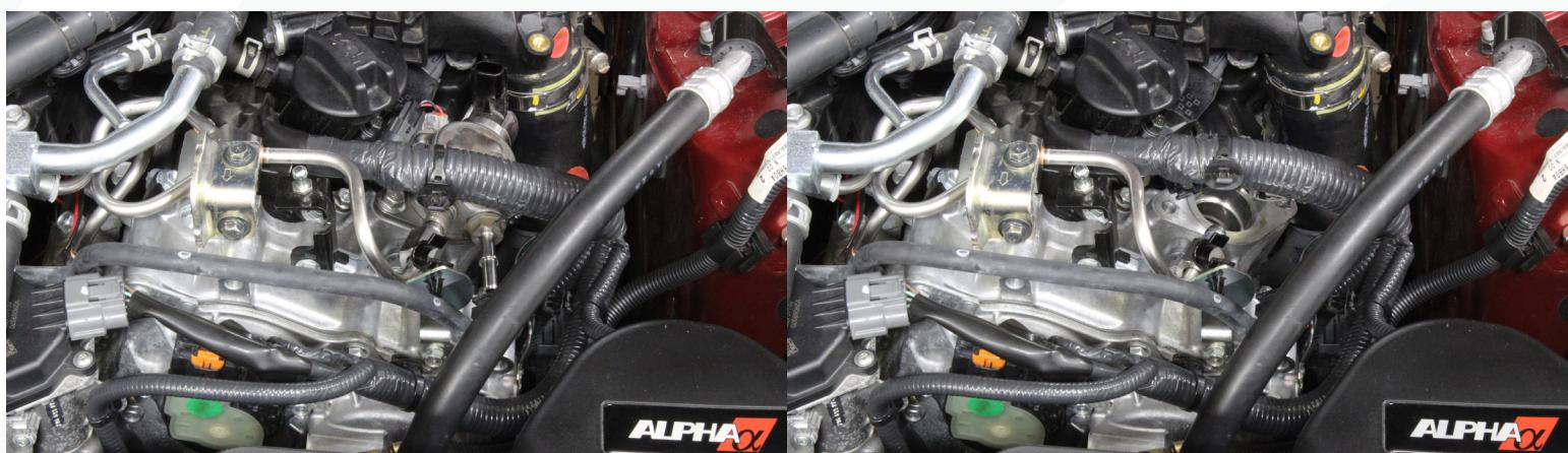
7) Make sure the surface of the cylinder head flange is clean. The OEM HPFP seals internally with an O-ring and the new AMS HPFP seals on the surface of the flange with an O-ring installed in the base plate of the HPFP.
