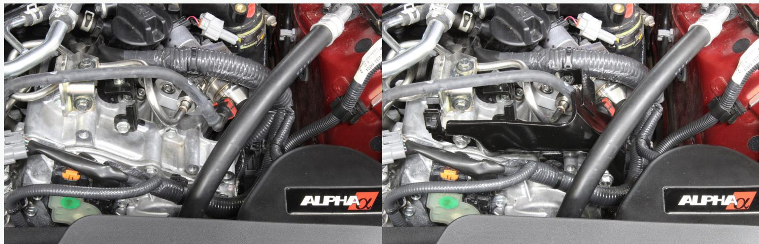
17) Double check all your connections. Reinstall the #52 (15A) fuse removed in the pressure relieving section. Prime and start the engine. Check all lines and fittings for leaks. Reinstall the engine cover once complete.
