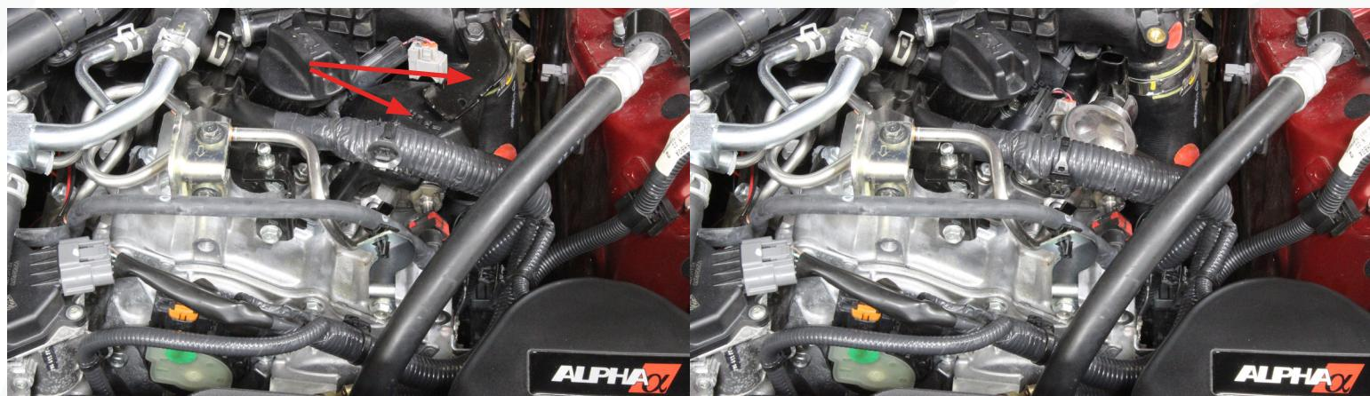
4) Make sure fuel pressure has been relieved as was explained in the first section of the instructions, and the engine is cool. Place a rag under the inlet and outlet fitting on the HPFP to catch any fuel left over in the lines. Start by releasing the red lock tab on the low side inlet fitting. Make sure not to force the red lock tab off as it could break. Carefully spread the two tabs at the top outwards and slide the lock tab downwards. Disconnect the fitting from the HPFP.
