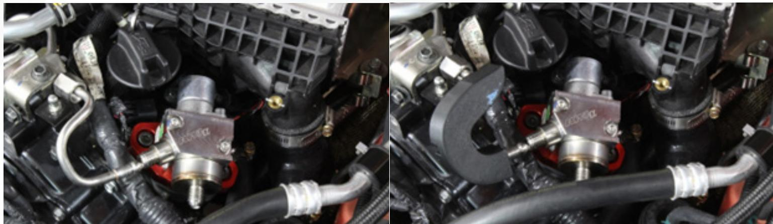
13) Once everything is lined up properly, install the two supplied M8 allen bolts. Make sure to tighten the bolts in steps the same way as was done during removal. Tighten the allen bolts to 22 ft lbs (29.5 N.m). Once the HPFP is torqued into place, tighten the high pressure fuel line coupler. Tighten the coupler nut to 27 ft lbs (36 N.m). Last, unbolt and retighten the high pressure line support bracket to take any unwanted stress off the line after the HPFP and fittings are tight.
