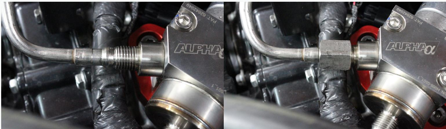
14) On the STAGE 1 HPFP, reconnect the low pressure line and slide the red lock into place. A little silicone spray is recommended on the fitting to prevent damage to fitting O-rings. There is a support bracket that can be removed since the low side line location changes with the HPFP.
