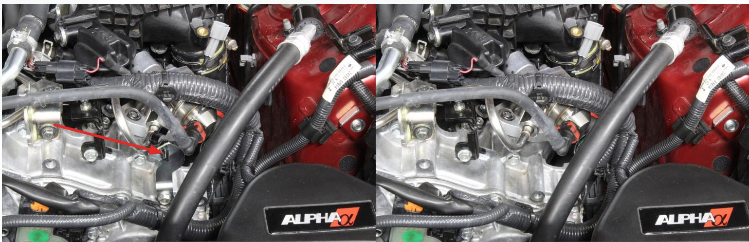
15) On the STAGE 3 & 4 HPFP, the inlet fitting is a -6AN male fitting. The OEM plastic feed hose does not have the correct fittings. There are 3 options listed below for a low pressure feed hose,
