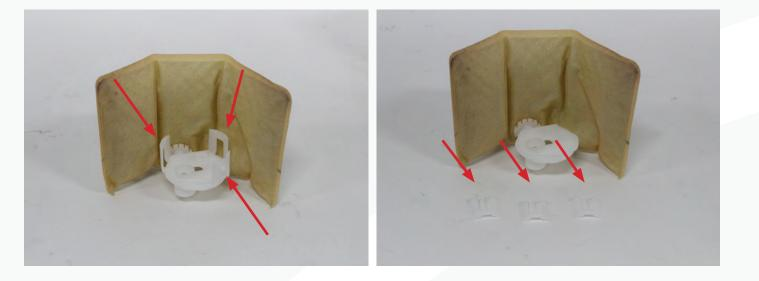
**26.** Locate the AMS fuel pump bracket supplied in your kit. Note how the pump bracket fits onto the filter.
