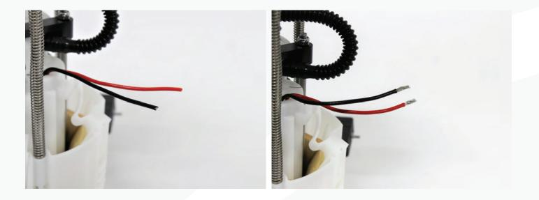
**36.** Make the connection between the harnesses with the supplied blue heat shrink sealed crimp connectors. Blue wire is connected to Red, Black wire to Black.
