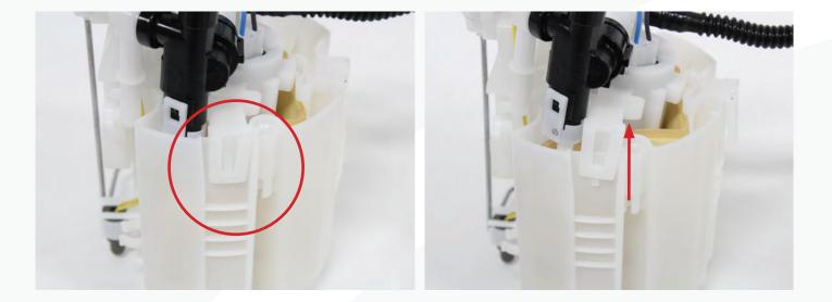
**16.** Remove the pump assembly from the sending unit basket.
