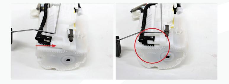
**34.** Cut the factory pump wiring about 2 inches from the white/clear pump connector. Strip the insulation from the ends of the blue and black wires on the harness remaining in the pump assembly by about 3/16".
