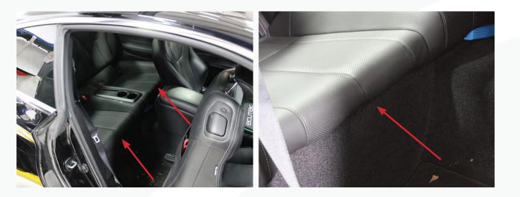
**2.** With the seat cushion removed, locate the fuel pump sending unit cover on the right hand side of the vehicle. Pull back and move the sound deadening cover to the side.
