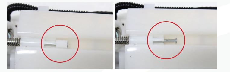
**12.** Release the tabs on both sides of the sending unit to release the spring loaded mounting rods.
