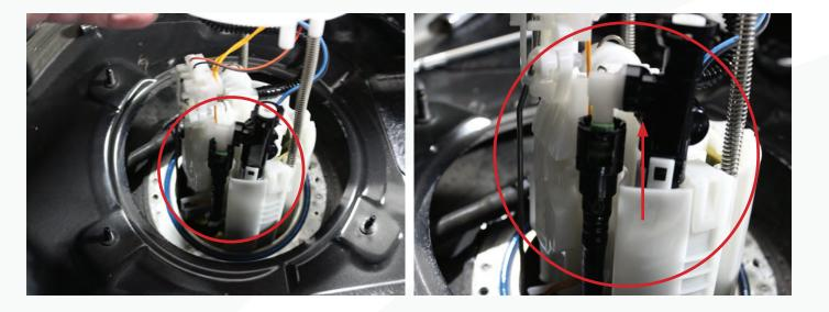
**40.** Fully seat the sending unit into the fuel tank, making sure the siphon hose is clear of the level sender and not routed underneath the sending unit. Reinstall the retaining ring, securing the sending unit in the fuel tank. The new unit is slightly taller than factory, so the unit will need to be compressed. Tighten the 6 M5 bolts (8mm wrench) securing the fuel sending unit.
