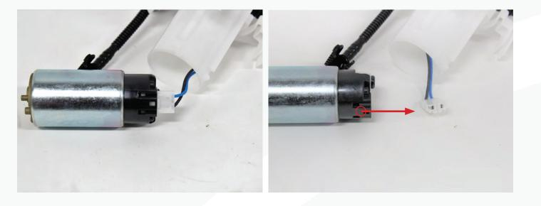
**20.** Check to see of the pump outlet O-ring removed with the pump, if not, it will still be inside the pump assembly housing. Remove the O-ring and set it to the side.
