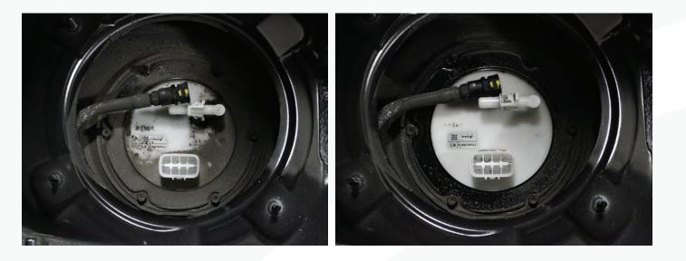
**8.** Remove the 6 M5 bolts (8mm wrench) securing the fuel sending unit and remove securing ring.
