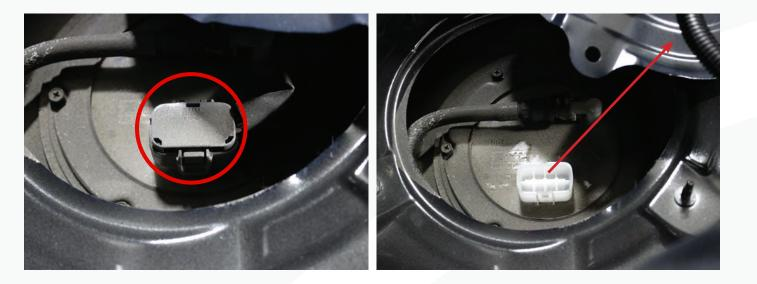
**6.** Make sure the fuel pressure has been relieved. Then disconnect the fuel hose connection on the top of the sending unit. Cover the connection with suitable rags to prevent fuel spray and to collect remaining fuel which may drain from hose.
