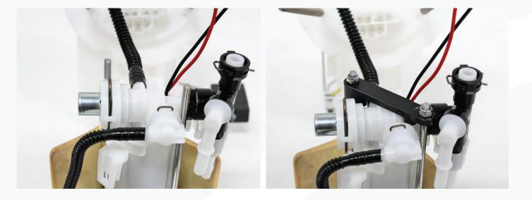
**29.** Reinstall the pump assembly into the sending unit.
