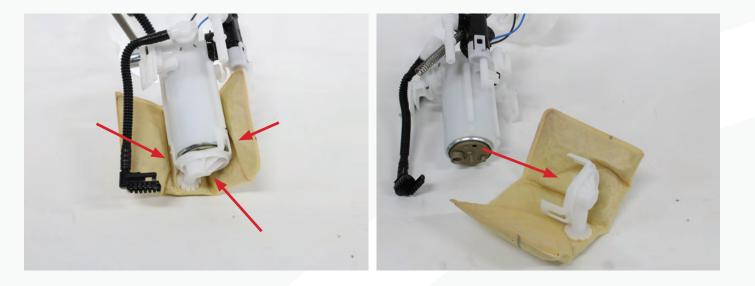
**18.** Remove the pump from the pump assembly.
