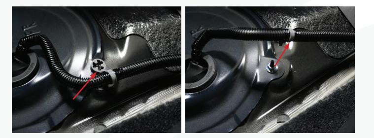
**4.** Remove the fuel pump sending unit cover by removing 3 - M6 nuts (10mm wrench).
