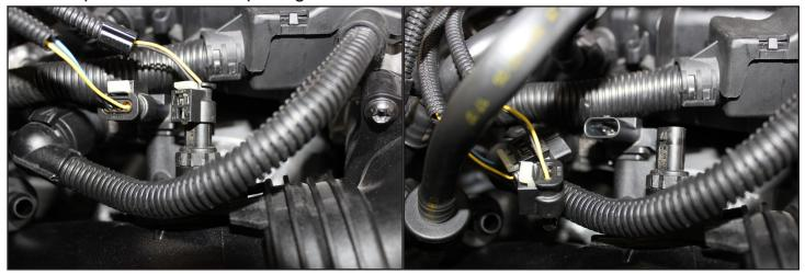
8. Remove the spring clip on the compressor outlet and pull the charge pipe toward the front of the car.
