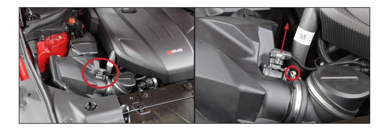
2. Release the four metal clips to remove the upper air box.
