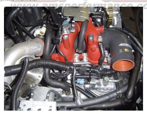
4. Install the intercooler pipe from turbo silicone outlet to the passenger side inner fender (leave bracket loose). Re-position horn if needed.
