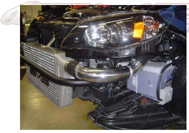
8. Install the next intercooler pipe that goes right next to the battery (it's two 45 degree pipes welded together, the longer 45 degree piece faces upwards).
