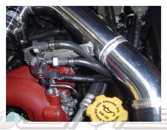
12. At this point a boost leak test should be done to ensure there are no leaks or loose connections. And also upon first start up check for any fuel leaks around the new fuel lines.
