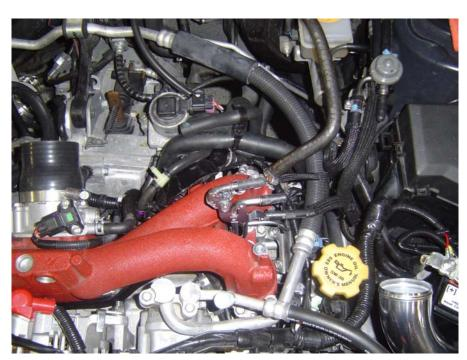
10. Install the blow off valve intercooler pipe and connect the vacuum line to the blow off valve. Bolt the intercooler pipe to the intake manifold with your factory hardware.
