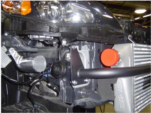
5. Install the second intercooler pipe. Now you can position the bracket from the first pipe and tighten it with the provided hardware.
