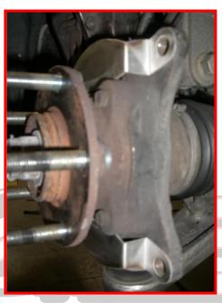
3. Reinstall the rotor. Install the included caliper duct adaptor while bolting the caliper back into place using the factory hardware. Using the supplied coated stainless steel reusable ties, secure the ABS sensor wire to the hub as shown to keep it from rubbing the rotor or touching the caliper (we ended up trimming about 1" from the length of the tie so it wouldn't rub the axle or CV boot).
