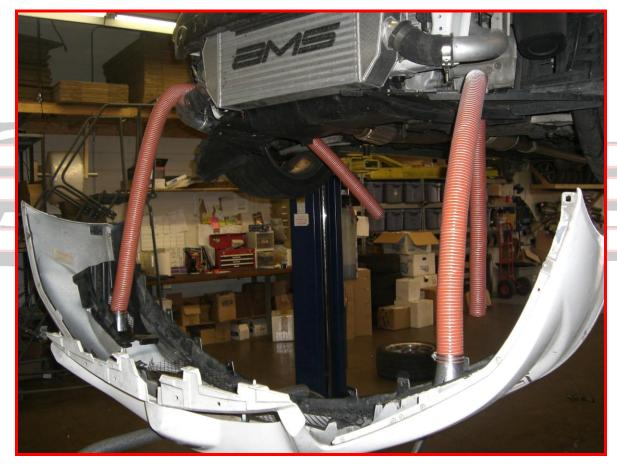
9. With the scoops in place, now you can run the hose through the engine bay and reinstall the bumper cover. To run the hose through the passenger side, most installs will require trimming the plastic oil cooler shroud. The factory undertray will also need to be trimmed to allow the hoses to reach the calipers. Make sure to zip tie the hoses effectively to keep them from touching any moving components (A/C compressor pulley, axles, control arms, etc) and away from very high sources of heat.
