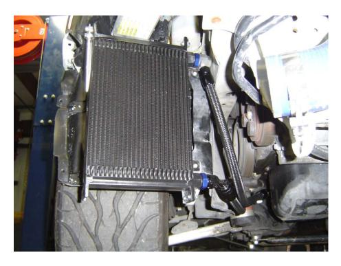
7. Make sure all fittings and connections are tight and check for leaks before driving.
