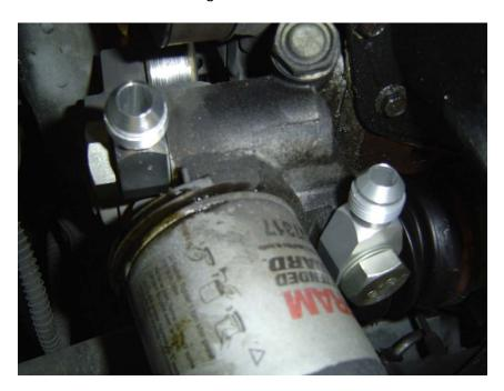
6. You can now install the oil cooler back onto the car and connect the lines to the oil filter housing. The longer line goes to the driver side fitting and the shorter line with the straight fitting goes to the passenger side fitting.
