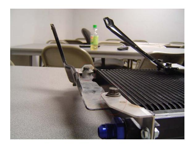
4. You can now install the lines onto the oil cooler as shown, you will want to tighten the top (longer) line before final installation, once installed on the car the line can be very difficult to get to.
