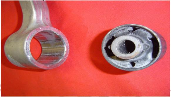
9. Coat the outside of the Delrin Bushing with lubricant (i.e. white grease, petroleum jelly. Wheel bearing grease)
