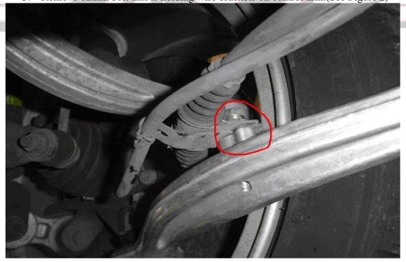
4. Remove 19mm bolt on the front of the control arm.(See Figure 3)
