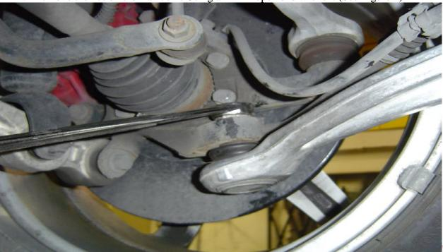
3. Remove 12mm bolt that is holding wire brackets on control arm.(See Figure 2)
