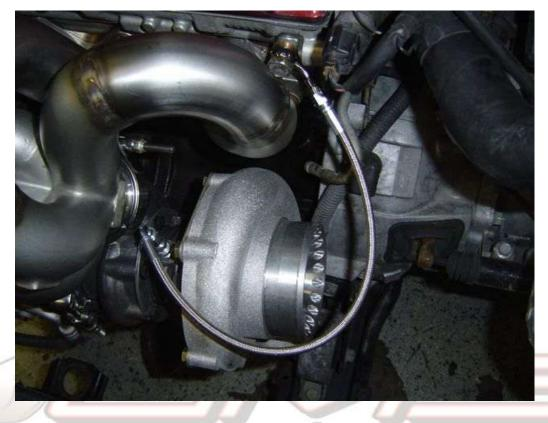
7. Loop the coolant lines using the supplied silicone hose.
