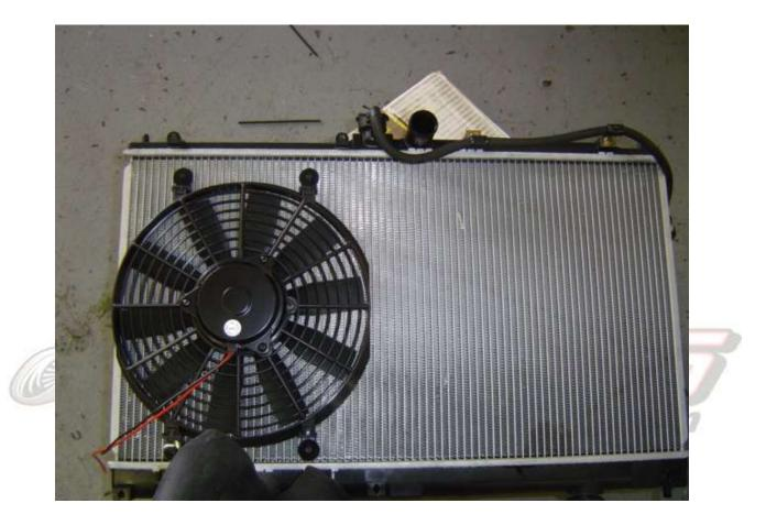
9. Install radiator and re connect fan and resistor box. Use the supplied heat wrap on the upper radiator hose and overflow hose. The overflow hose also gets re-mounted using the supplied clamps that fit over the heat wrap. If the radiator hose is too close to the exhaust manifold you can cut off 1-1.5" off the radiator end of the hose to pull it away.
