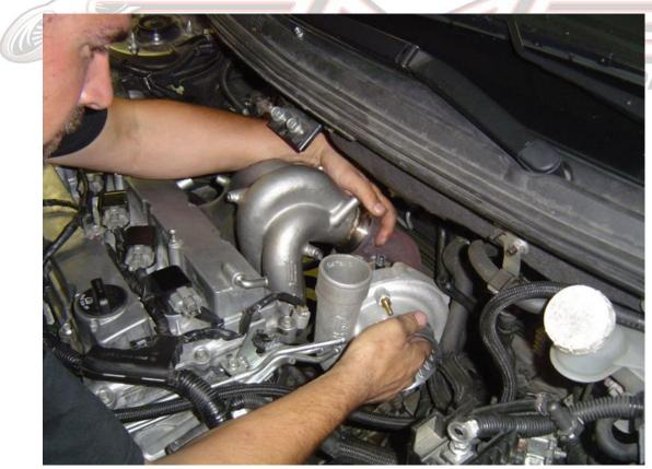
14. Take a look at the support bracket where it bolts to the factory bracket. IF there is a space in between the two this space must be filled with the supplied thick M12 washer, this must be done to ensure the support bracket will not be getting pulled down. Install the nylock nut and bolt at bottom of support bracket to hold the assembly in place. Leave loose for now to allow movement of the turbo.
