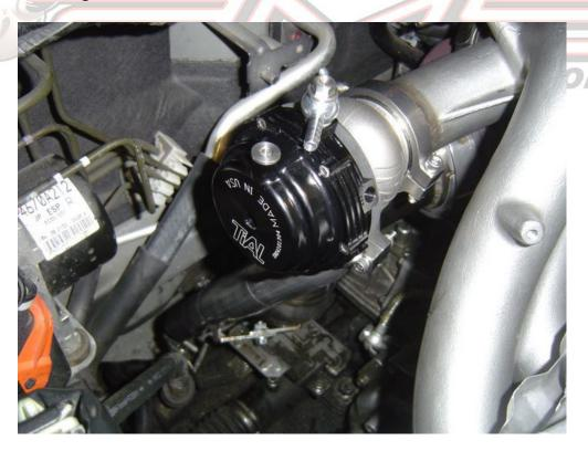
20. Loop turbo coolant lines. (Don't do this if you bought the optional wastegate water cooling kit.
