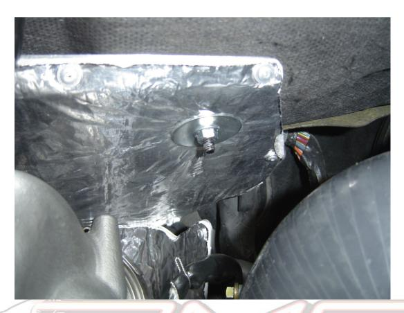
23. Install manifold shield.
