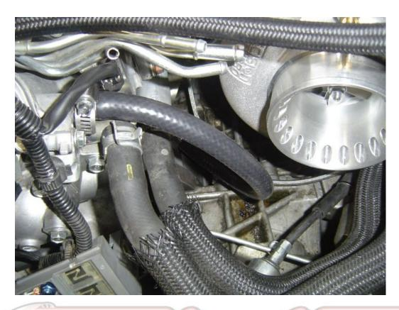
21. Install supplied heater hose on AC line that is on the firewall.
