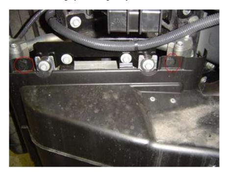
9) At this point you can remove the factory intercooler piping and install the AMS kit as shown below. We have found that when installed as shown the kit fits very well on most cars, in some rare cases fitment is found to be better by flipping the mid and lower pipes. Install the kit so it fits your particular car best. Some things to keep in mind during install are clearance around oil cooler and radiator shroud, and clearance from the wheel wells.
