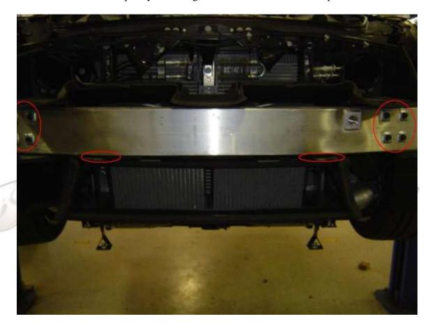
8) Remove oil cooler ducting by removing 4 clips.
