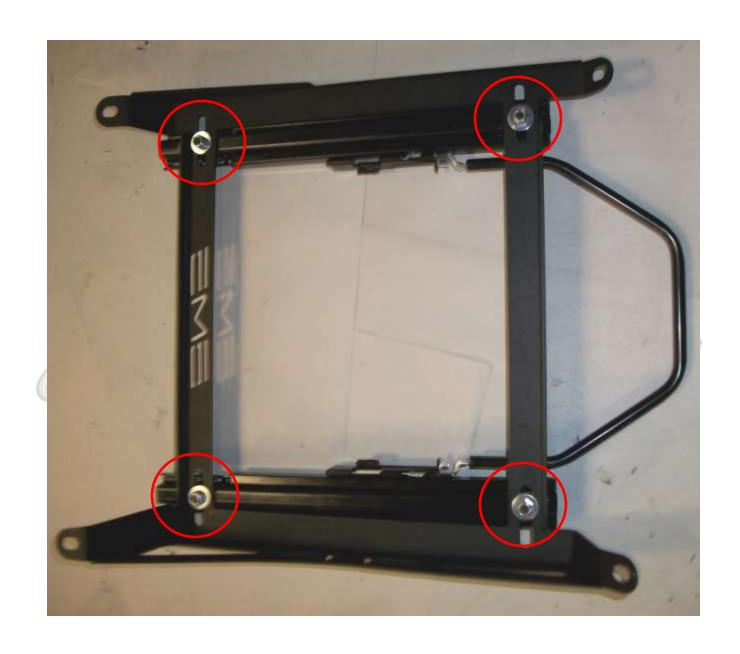
2. Next, install the Seat Mounting Brackets onto the Sliding Tracks (as pictured in "Side View" noting "FRONT" with the curved area closest to the rear of the Seat Base) using 4 Hex Head Bolts with 4 Large Flat Washers on top ("Top View 2" yellow circles) and 4 Small Flat Washers with 4 Nylon Lock Nuts on the bottom ("Bottom View 2" close-up). Do not tighten hardware until final fitment has been figured out.
