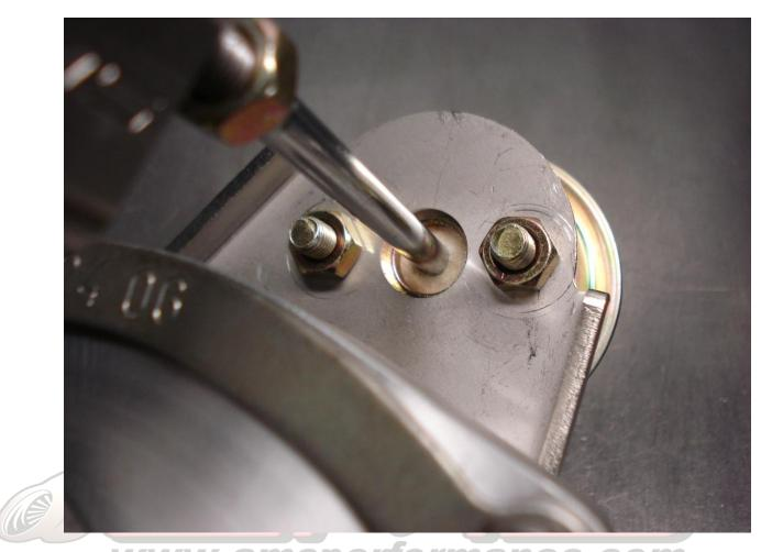
As an extra step to ensure there is no binding in the assembly you can use compressed air to move the WGA. With a regulator set at 0 PSI connect it to the WGA nipple, then slowly and gradually raise the pressure until the WGA arm begins to move (~15 PSI), making sure it's at your desired boost level. Tighten the jam nut on the other side of the arm, making sure the preload doesn't change.
