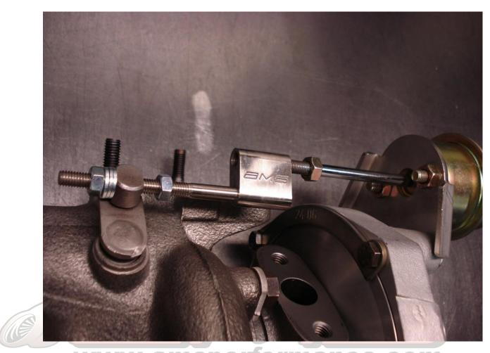
5) Now set the preload. Measure the length of the WGA rod that is sticking out from the end jam nut in millimeters (yellow line). Now tighten the nut until there's an additional 1-2mm which is the recommended starting point.
