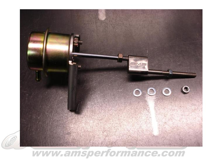
3) Position the AMS WGA on the turbo with the rod going through the eyelet on the arm, then bolt the bracket to the compressor cover with the supplied M6 bolts.
