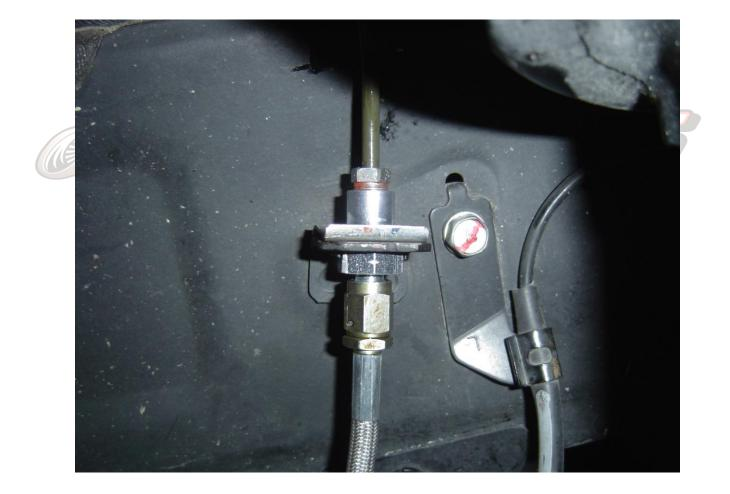
8. Install the brake lines and route them as shown in the picture and hold in place using factory clips.
