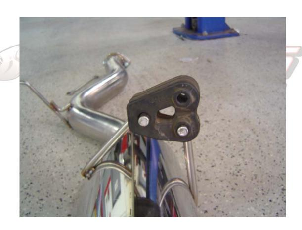
3) At this point you can hang the rear section onto the car.
