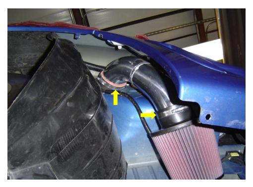
c) Use existing stud and nut shown and loosely hang cold-air intake pipe.
