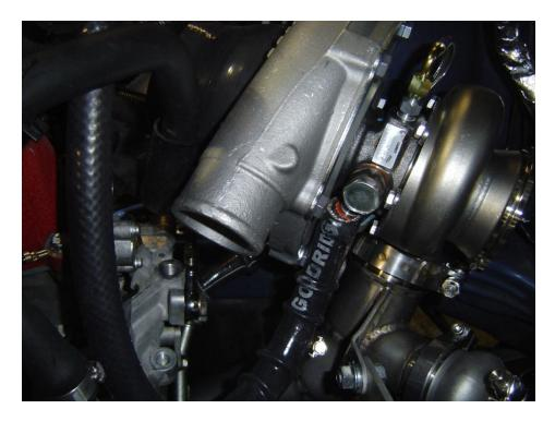
10) Install the 90° end of the oil feed line on the turbo, routing it around the passenger side. Tighten both sides of the line. **NOTE:** BE CAREFUL NOT TO OVER-TIGHTEN AND STRIP THE ALUMINUM OIL FITTINGS ON EITHER SIDE OF THE LINE!
