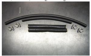
10mm turbo coolant lines with heat sleeves
