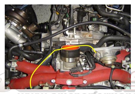
i) Make sure all turbo intake pipes, hoses, and lines are routed properly and then tighten all the clamps and double-check all your connections. Bolt cold-air pipe all the way down, then re-install inner fender well liner and wheel.
