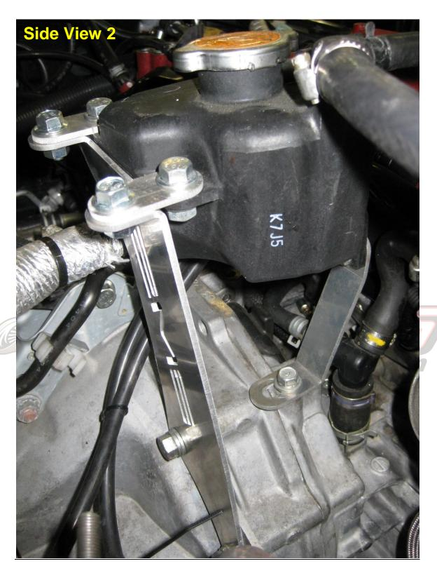
Install the brackets as shown with the large "AMS" one being stacked behind the turbo kit up-pipe support bracket on the transmission. Make sure to keep ALL lines away from any sources of high heat and/or abrasion using protective heat sleeve where necessary.
