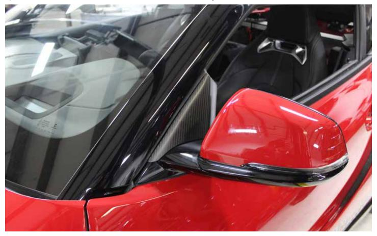
**3)** Clean off the mirror base with isopropyl alcohol and let dry. It is very important that the surface of the mirror is clean before installing the plates.
