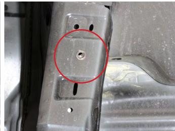
7. Once the rivet nut is installed, install the tank and secure the front bracket with the M8 stainless bolt as shown. contaminants into fuel tank..
