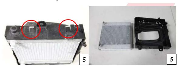
6) Install the new Alpha heat exchanger into the shroud in the reverse order.
