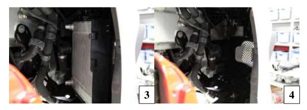
5) To remove the cooler from the shroud, release the tabs on the bottom and top of the shroud shown in the picture.
