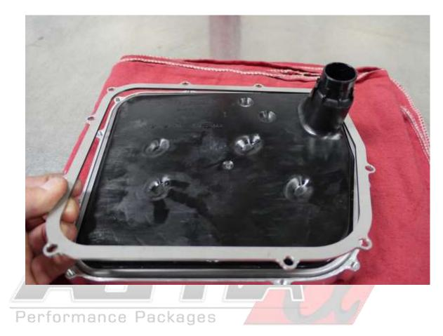
8. Flip pick-up assembly over. Install included allen cap screws with washers into the threaded holes(4). Use high temp/strength thread locker. Torque to 90 in/lb
