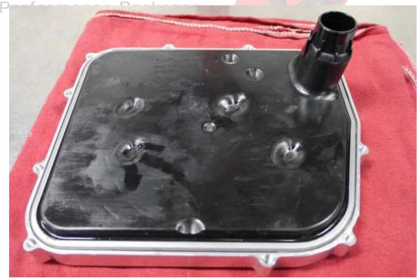
Install Alpha retaining ring as shown using the included M6 button head screws. Use high temp/strength thread locker. Torque to 90 in/lb
