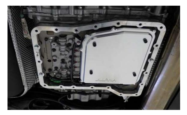
15. Install factory transmission oil pan with sealant (we recommend Three Bond #1217H) using the included M6x30mm bolts. Discard the factory gasket. Torque to factory specs.
