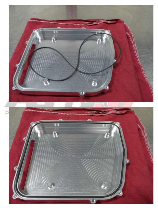
6. Install factory filter/pick-up into the Alpha billet housing as shown. NOTE: The fit is tight and may require some light force to seat it all the way into the pickup. Also, it is important that the o-ring stays in its seat/groove.
