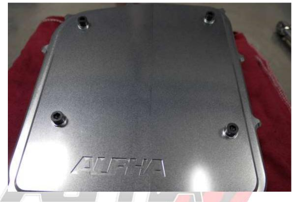
9. Clean sealing surface of transmission. Make sure no fluid/dirt remains.
