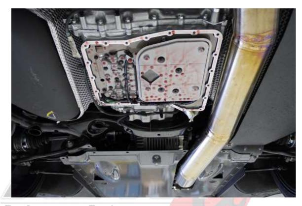
4. Carefully pry/slide the factory filter/pickup straight-down to remove it from transmission.
