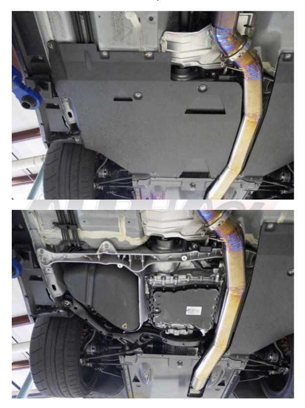
1. Lift vehicle and remove under tray that covers transmission.
