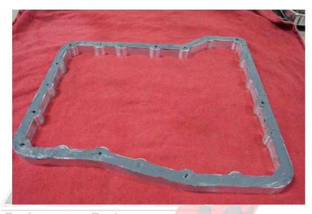
11. Install spacer onto transmission using included M6 bolts. Snug the spacer onto transmission to set sealant. Wait at least a half an hour to let the sealant cure enough to hold the weight of the spacer.
