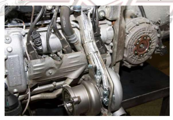
27) Next use the stainless steel ties to attach the lines to the support bracket. Make sure all the lines are as low as possible.
