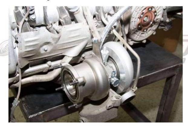
24) Next get the longer oil feed line and install. Route it on the right side of the support bracket then under the fuel rail to the oil feed port on the front of the cylinder head where you installed the gold billet oil feed fitting.
