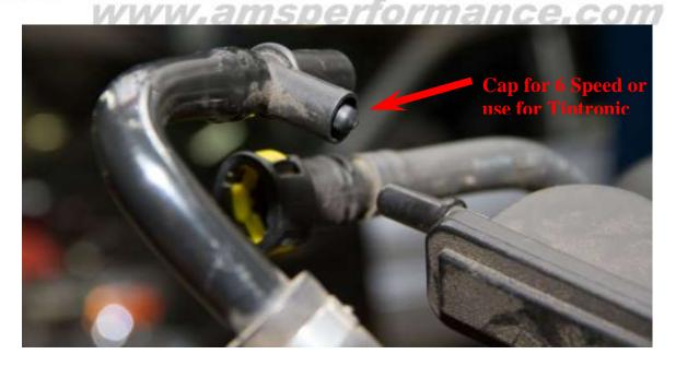
13) You can also remove the plastic line that runs from the bottom of the solenoid to the brake boost line. Use the supplied 1/8" vacuum cap to cover this port shown in the illustration for 6 speeds cars.
