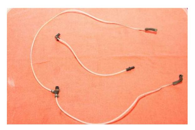
12) Remove the white plastic air tubes running from the factory turbo bypass valve to the control solenoid. The lines can be removed but the solenoid will remain in place and plugged in to avoid and check engine lights. Boost control must now be done by an external controller and will be covered latter in the install.
