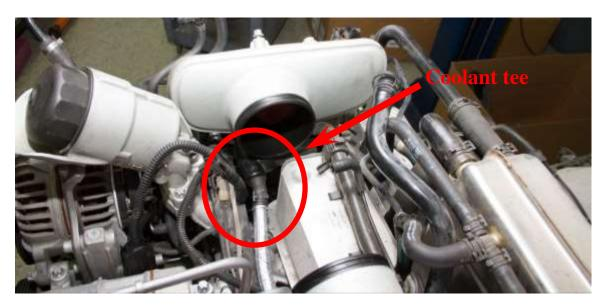
26) Next route the other coolant line that was already installed on the turbo over the top of the fuel rail to the factory coolant distribution tee. Use the factory clamp.
