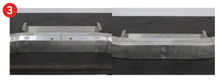
**4.** Set the crash beam in front of the intercooler installed on the vehicle to make sure your marks are correct.
