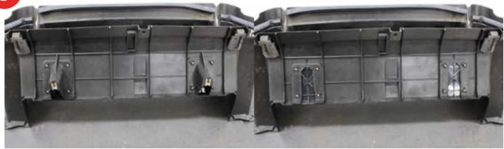
**4.** Trim off as much of the webbing under the duct as shown. This will allow the duct to flex around the intercooler.
