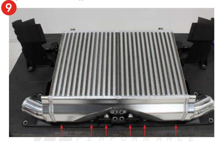
**10.** In the hardware kit locate the two red support brackets. Install the brackets with the supplied M6 and M10 hardware. Leave loose for the moment as final adjustments will be made when installed on the car. Make sure the bracket with the small square cut hole in installed the right side / passenger side of the car. This hole is for the outside air temp sensor.
