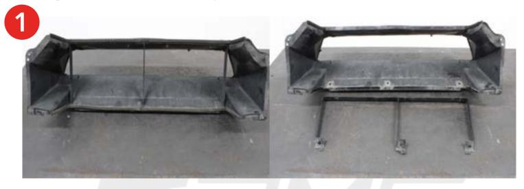
**2.** Trim the top section of the air duct as shown in the picture below. Make sure to leave about 1" at the area shown in the second picture.
