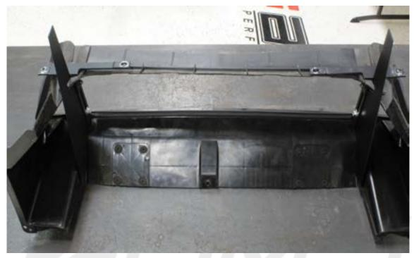
**8.** Use the supplied foam strip and apply it to the bottom of the duct shown. Skip the area in the center shown.
