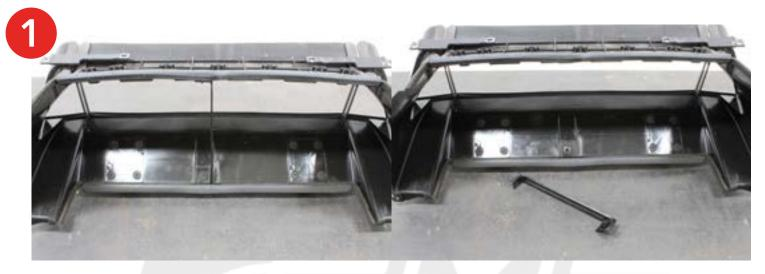
**2.** Trim the top section of the air duct as shown in the picture below. Make sure to leave about 1" at the area shown in the second picture.
