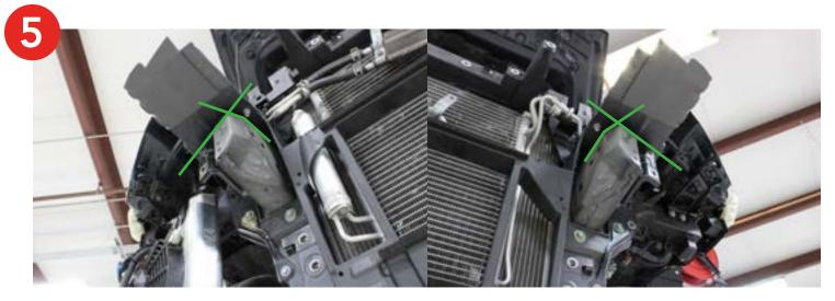
**6.** Remove the support and highlight the marked area shown using your traces. This area needs to be cut out. The after pictures are also shown below.
