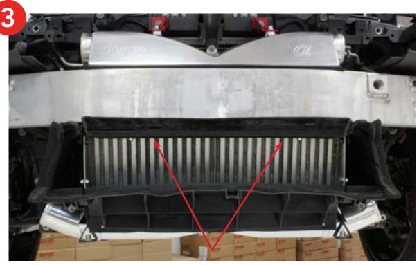
**3.** Locate two small aluminum horn brackets. Remove the factory bracket off the back of the horns. Using the original hardware, install the new brackets leaving them loose for final adjustment. The horns do have different tones and have to be installed on the original sides. Install the horns and bend the brackets as necessary for fitment.
