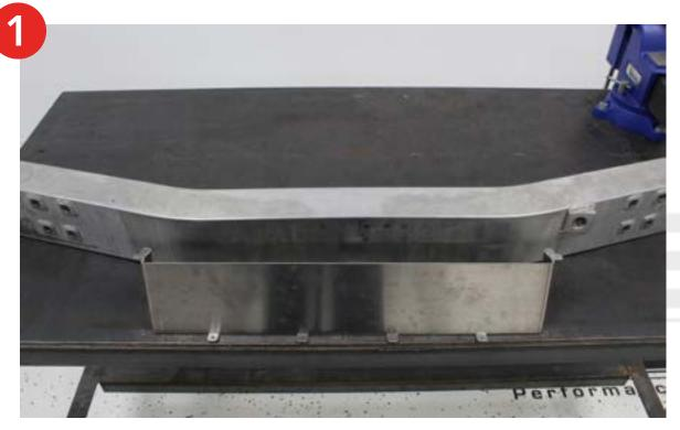
**2.** Start by placing the patch panel over the rear of the crash beam and marking it. Make sure it is centered on the beam.
