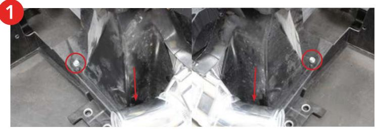
**2.** Reinstall the core support and intercooler assembly back onto the car. It can be permanently installed. Make sure to lift the intercooler support as high as it will go before tightening. The weight of the intercooler will pull down on everything slightly. If this is not done, the bumper and hood alignment will be off.
