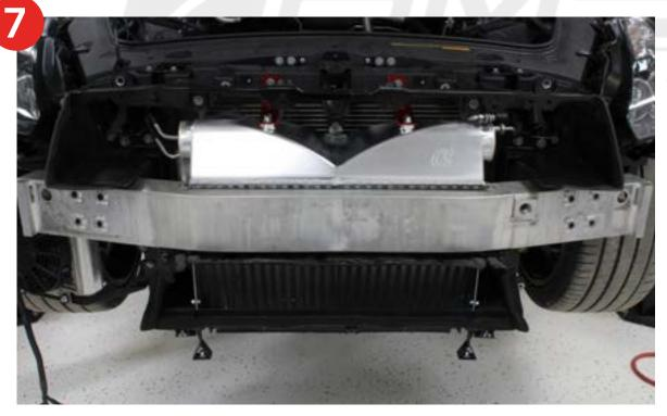
**8.** Adjust the intercooler upper brackets if need be. The entire intercooler support can also be moved around to center the cutout area on the intercooler if need be.
