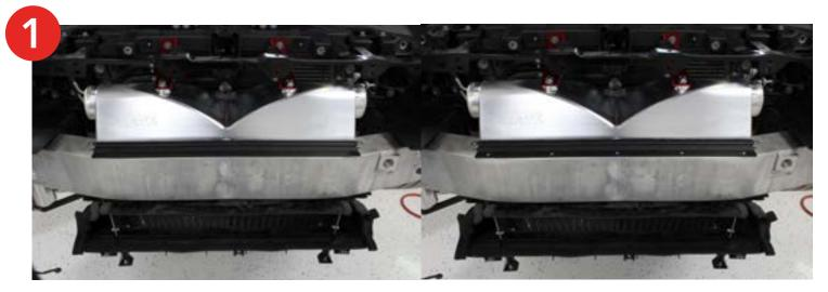
2. Install the factory hardware in the outside holes of the lower lip support brackets. Line up where the inside holes are on the plastic air duct and drill a ¼" where the mark is. Locate the lower plate air duct plate. I will have two ¼" holes and a small bend. Install the plate with the hardware shown below in the order shown. The bend will be facing towards the intercooler and pointing upwards. Order (Bolt, Plate, Air Duct, Washer, Spacer, then bolted into the core support)
