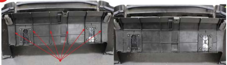
5. Trim off the bottom section of the lower air duct up to the rivets as shown
