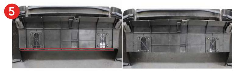
**6.** Next cut 2 slits in the lower part of the duct. No material will be removed in this step. The slits allow the duct to lex to a new pro ile. Only cut the area shown, do not over cut this area. Trimming in a later step may be needed. Note: Side shrouds for both model year breaks included
