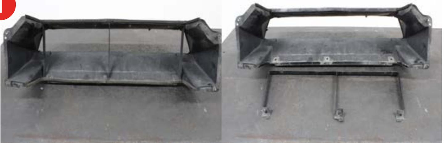
2. Trim the top section of the air duct as shown in the picture below. Make sure to leave about 1" at the area shown in the second picture.
