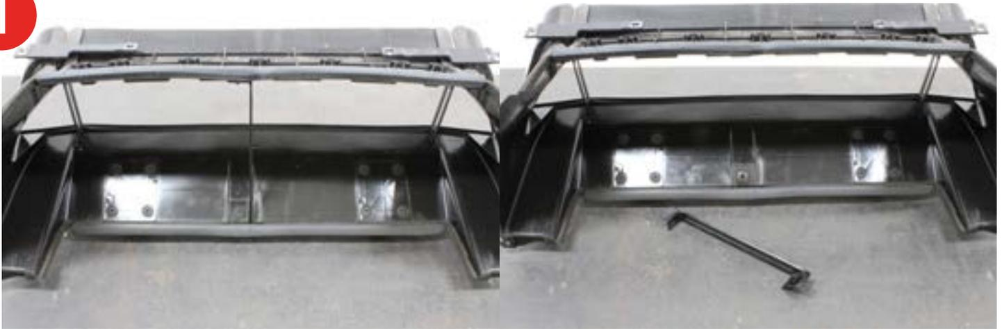
2. Trim the top section of the air duct as shown in the picture below. Make sure to leave about 1" at the area shown in the second picture.
