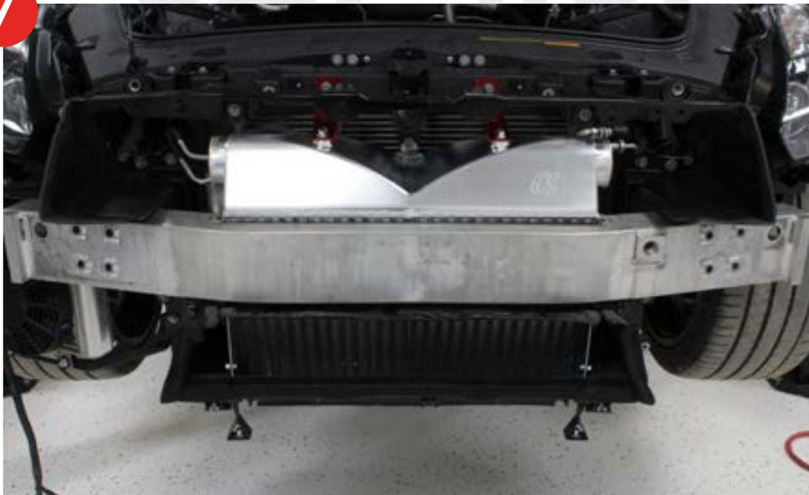
8. Adjust the intercooler upper brackets if need be. The entire intercooler support can also be moved around to center the cutout area on the intercooler if need be.
