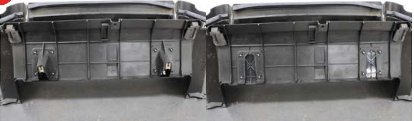
4. Trim off as much of the webbing under the duct as shown. This will allow the duct to flex around the intercooler.
