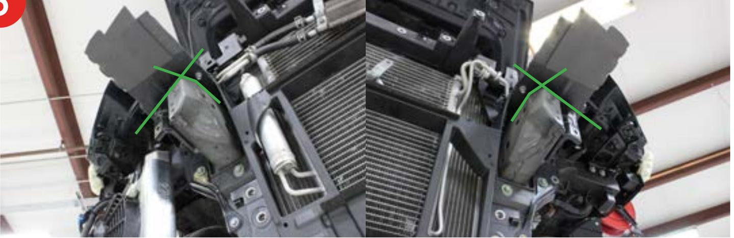
6. Remove the support and highlight the marked area shown using your traces. This area needs to be cut out. The after pictures are also shown below.
