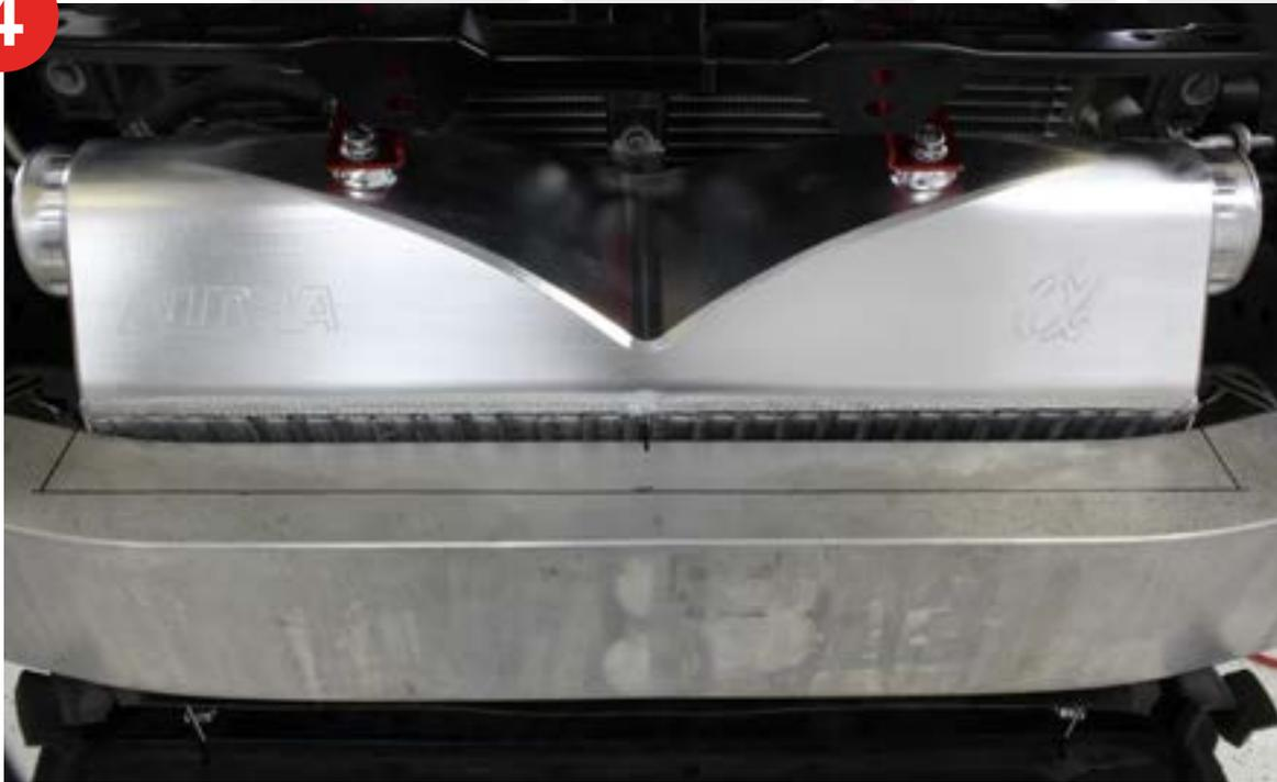
5. Cut the crash beam. Continue to cut and fit until the patch panel fits perfectly into the crash beam. Use any means to fit the panel, (band Saw, cutoff wheel, mill). The panel will need a little manipulation around the extruded sections of the beam as they are not flat.
