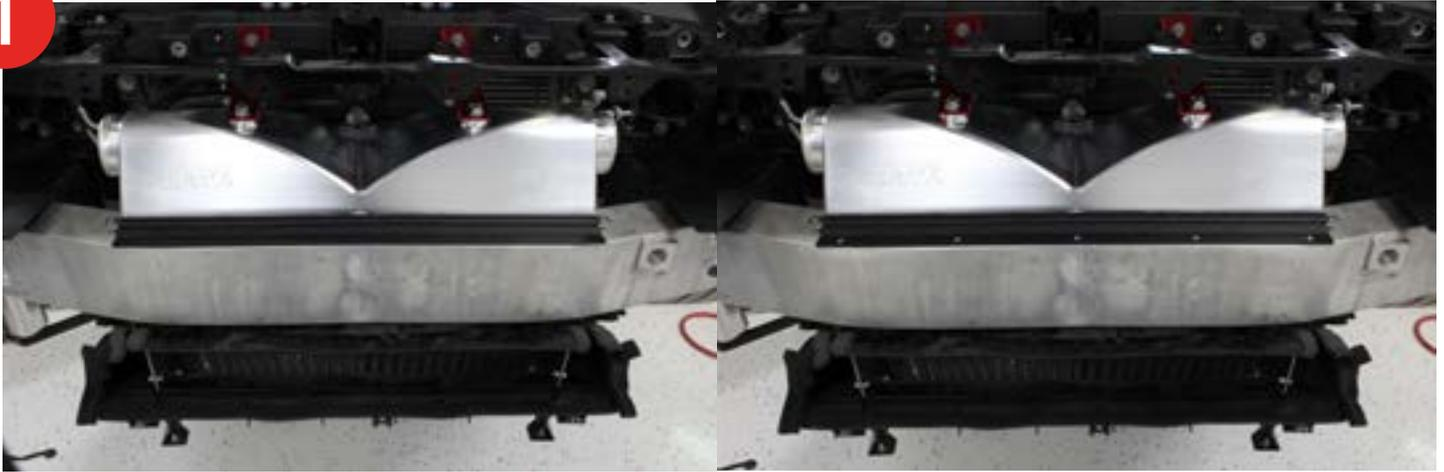
2. Install the factory hardware in the outside holes of the lower lip support brackets. Line up where the inside holes are on the plastic air duct and drill a 1/4" where the mark is. Locate the lower plate air duct plate. It will have two 1/4" holes and a small bend. Install the plate with the hardware shown below in the order shown. The bend will be facing towards the intercooler and pointing upwards. Order (Bolt, Plate, Air Duct, Washer, Spacer, then bolted into the core support)
