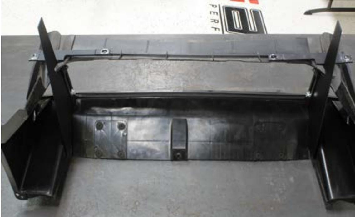
8. Use the supplied foam strip and apply it to the bottom of the duct shown. Skip the area in the center shown.
