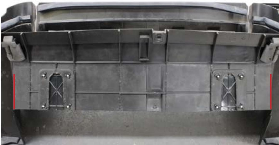
7. Install the supplied side plates and factory lower lip support brackets. Use the supplied hardware to install the side plates. The side plate lower profile will push and form the lower part of the air duct downwards. Trim more if needed as down in step # 7 to get the plate and profile correct
