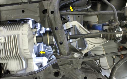
8. Secure the hose to the filler neck hose with the supplied zip ties and connect the hose to the barb fitting on the bottom of the overflow tank with the supplied worm clamp. Trim hose if needed.
