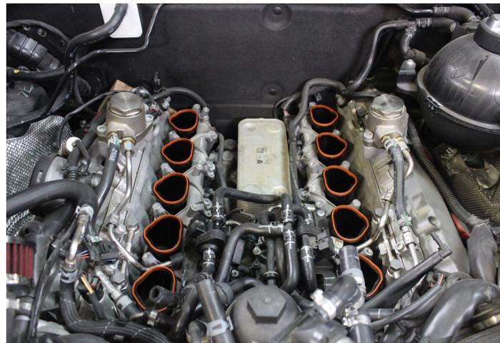
9. Install the intake runner gasket retainers on each runner. The notch on the underside will fit into the groove on the lower intake manifold runners.
