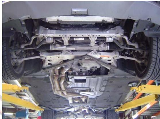
2. Pull back on both of the spring clips holding the intercooler piping to the intercooler. Then disconnect the piping from the intercooler.
