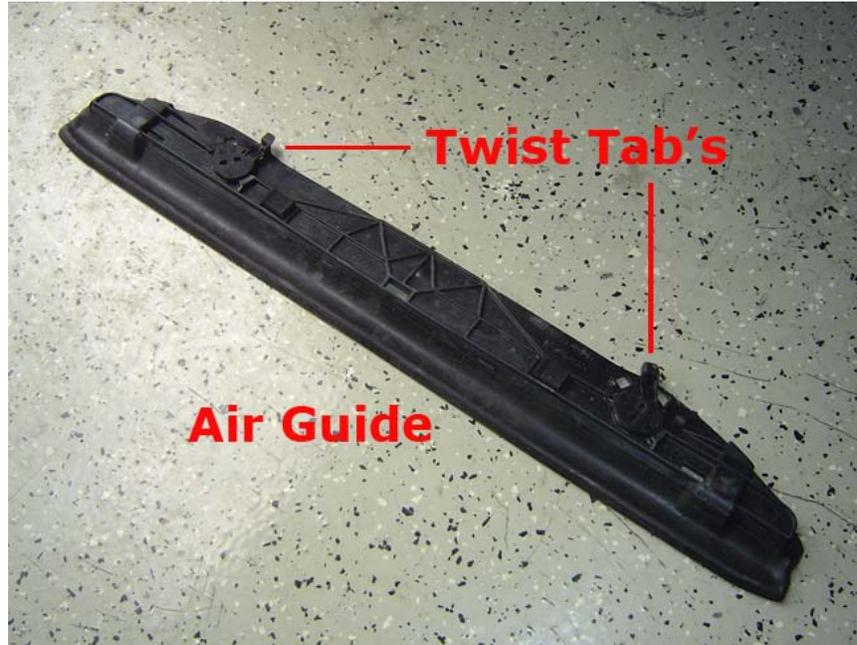
4. Twist the tabs and disconnect the fan shroud from the intercooler.
