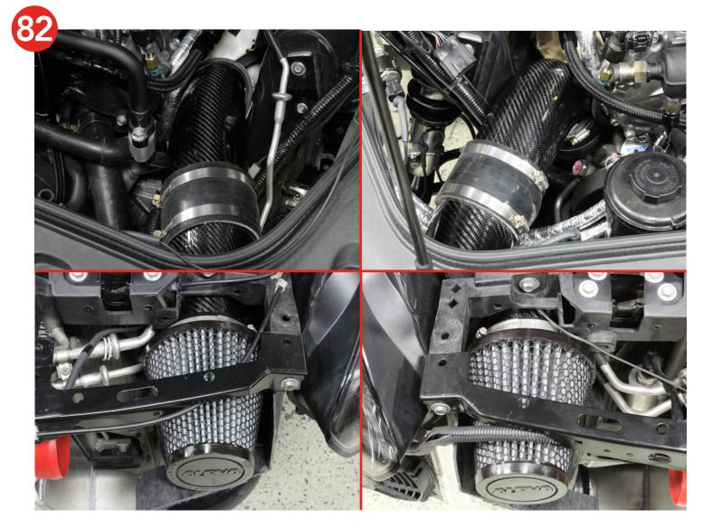
Tech Note: The Alpha air filters may look small, but offer extreme flow. They were designed especially for this turbo kit and are packed with the same amount of filter media of a conventional aftermarket filter 3x its size. During testing, there was only a .2psi pressure drop change @1400whp when removing the filter and netted no measureable hp gains. See the addendum at the end of the instructions for cleaning procedures.
