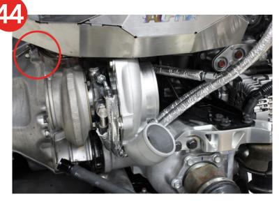
45. Install and tighten the -8AN oil drain on the right side.
