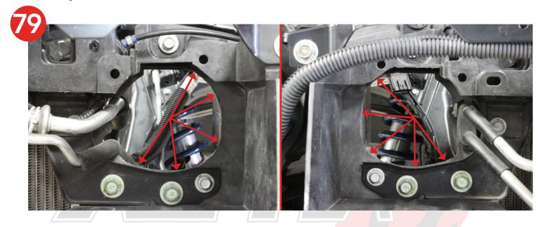
**80.** Test fit the carbon intake tubes with the filter. Remove more material if needed.
