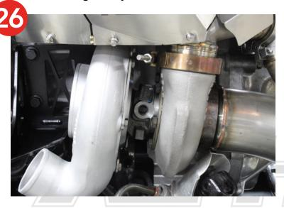
27. Locate the compressor outlet silicone, cast charge pipe, and hardware. Install the silicone and charge pipe as shown. Use the supplied M8 bolt, large washer, and aluminum spacer to bolt the charge piping to the factory location. Install the spacer between the cast charge pipe and the factory mounting bracket.
