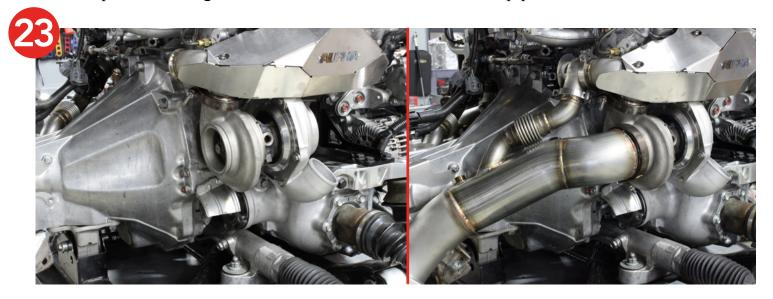
**24.** Install the mid-pipe you plan on using with this vehicle. Only snug down the mid-pipe bolts for now. Since there is slight adjustment in the turbo kit and variation between different manufactures of exhaust systems, doing this will help align the system as a whole.
