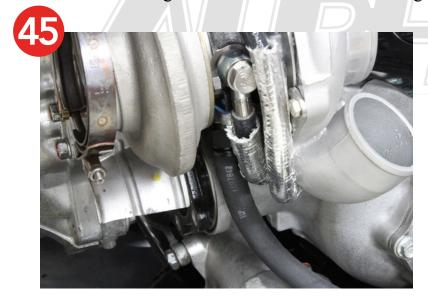
**46.** Make sure the factory banjo bolts for the water and oil feed fittings are used. The water fittings that are used in the side of the engine block are labeled with a W. The oil feed fittings that are used on the rear oil distribution block are labeled with an R. The R bolts are important as they are factory restricted and work in conjunction with the restricted banjo fitting installed on the turbos.
