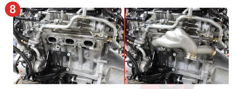
**9.** Repeat step (8) and install the right side manifold in the same manner. The third nut from the front will require an open 14mm wrench.
