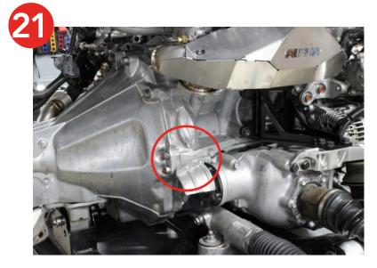
22. Locate the block shield from the heat shield kit. Install the shield as shown. Use a rubber mallet to foam the shield against the block where clearance was made. The shield will form easily to the block. Make sure there is a small air gap between the turbine housing and the block, otherwise, the direct contact will transfer heat.
