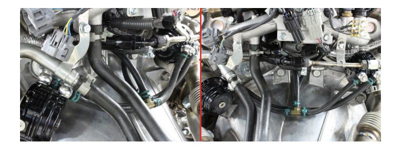
**68.** Once all your boost control lines are routed, use the supplied reflective heat wrap to cover all the lower silicone hoses including the clamps as shown in the pictures below.
