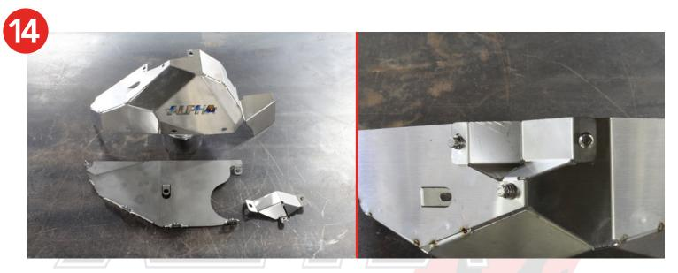
15. Remove the factory water pipe. Install the main shield onto the manifold. Leave the hardware loose for the time being. Install the plate under the bottom of the manifold. Last install the two small top heat shields on to the main shield. Start by tightening all the hardware on the manifold first, then finish by tightening the remaining hardware on the shields. Tighten the 10mm nut last on the rear of the shield.
