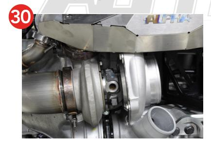
**31.** Locate the compressor outlet silicone. Install the silicone as shown. Clock the compressor cover downwards as much as possible leaving the smallest amount of clearance between the outlet silicone on the cover and the billet differential mount. There is also a picture of the silicone removed to see approximately how much clearance there is once adjusted. Again, adjust with the silicone installed and make sure there is enough room to get a hose clamp on as well.
