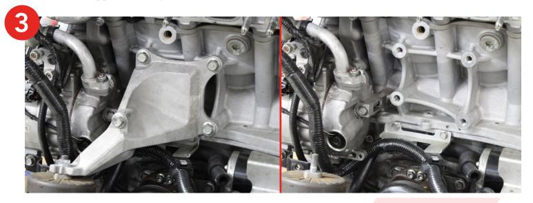
**4.** The factory motor mount stud needs to be trimmed slightly to add clearance for the compressor outlet silicone. Cut the stud down to the start to the threads if this has not already been done.
