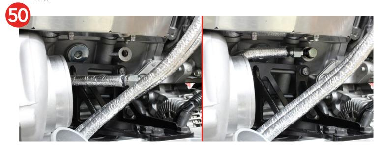
51. Route the oil feed and coolant line under the compressor cover and over the engine mount bracket as shown. Use a supplied metal tie to hold the lines in place. Route the lines up and over the manifold.
