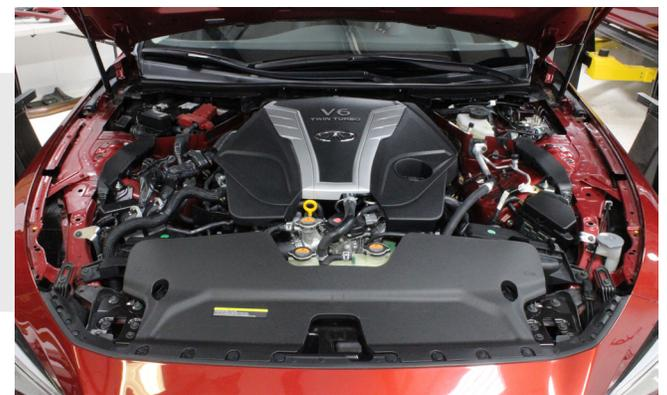
**3) Remove the front core support cover / air box inlet duct panel.**
