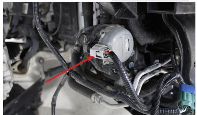
**23)** Route the remaining grey connector above the crash beam through a hole right below the headlight as shown.
