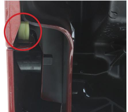
**10)** Just above the headlights where the top of the bumper and the fender meet, there is a 10mm bolt and retainer plate holding the two together. Remove the hardware shown
