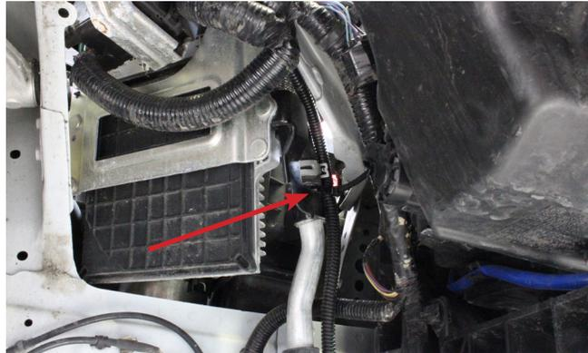
**27)** Undo the two 10mm bolts holding the ECU bracket and right side airbox bracket. Lift the two brackets and route the harness underneath them. Reattach the two 10mm bolts.
