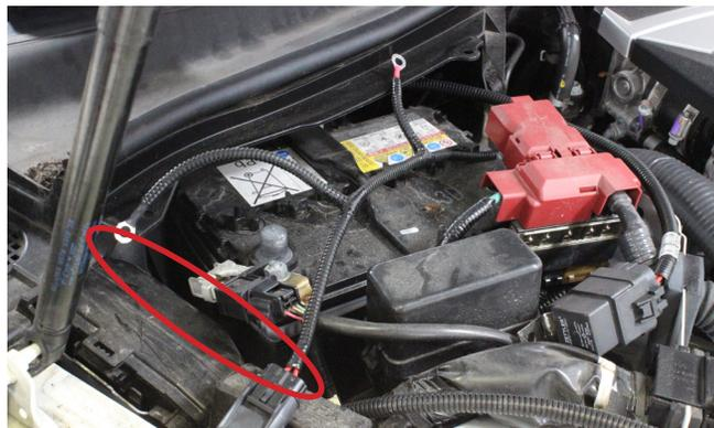
**29)** Loosely attach black and red ring terminals to the corresponding battery terminal by unscrewing the 10mm terminal nut. Attach the terminals back on to the battery. Orient black ring terminal pointing straight towards the back of the battery as shown. The red ring terminal must be angled down towards the battery and bent slightly to go in between the battery vents. A top and side view are given to show how to orient and bend the red ring terminal. Close the red plastic terminal cover.
