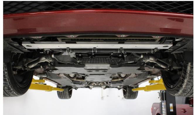
**5) Remove both front wheels and both front wheel well liners. You only have to remove the front half of the wheel well liner.**
