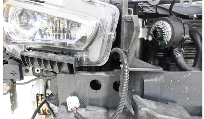
**24)** Feed the loom behind the plastic ducting by compressing the foam to get the loom up and over into the correct location.
