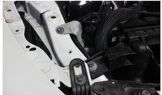
**28)** Route the relay end of the wiring harness around the battery in the battery box. Tuck excess harness length into the circled area to the left of the battery.
