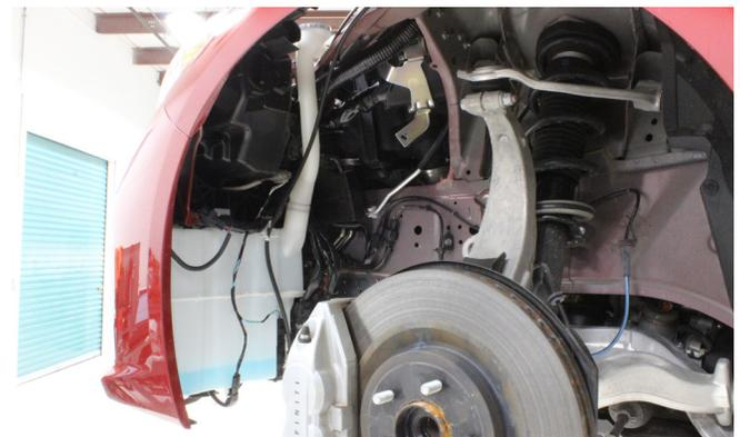
**6)** Disconnect the front LED running light harnesses on both sides. The connectors are located just below the headlights.
