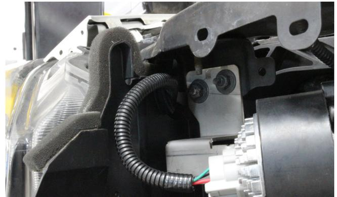
**25)** Position the harness as shown in the left image. Zip tie the harness in the locations shown with arrows. Ensure the harness has a little slack between zip ties. Orient the zip ties so that the head of the zip tie sits above the new harness loom.
