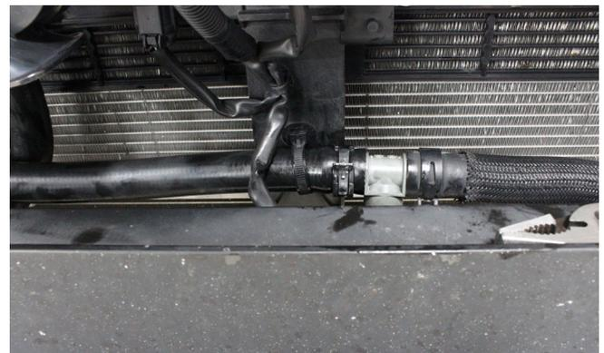
**18)** The remaining hose will have a 90-degree bend on one end and an obtuse angle bend on the other end. Attach the obtuse angle end of the hose to the fitting in the right wheel well area where the factory hose was previously removed. Use a hose clamp to secure it. Feed the other end of the hose through the gap in the factory plastic ducting shown.
