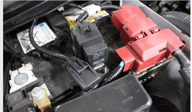
**32)** Reassembly of vehicle is opposite of the disassembly procedure. When replacing the battery box trim piece, ensure that the new harness is not pinched. Keep the new harness tight to the existing vehicle harness.
