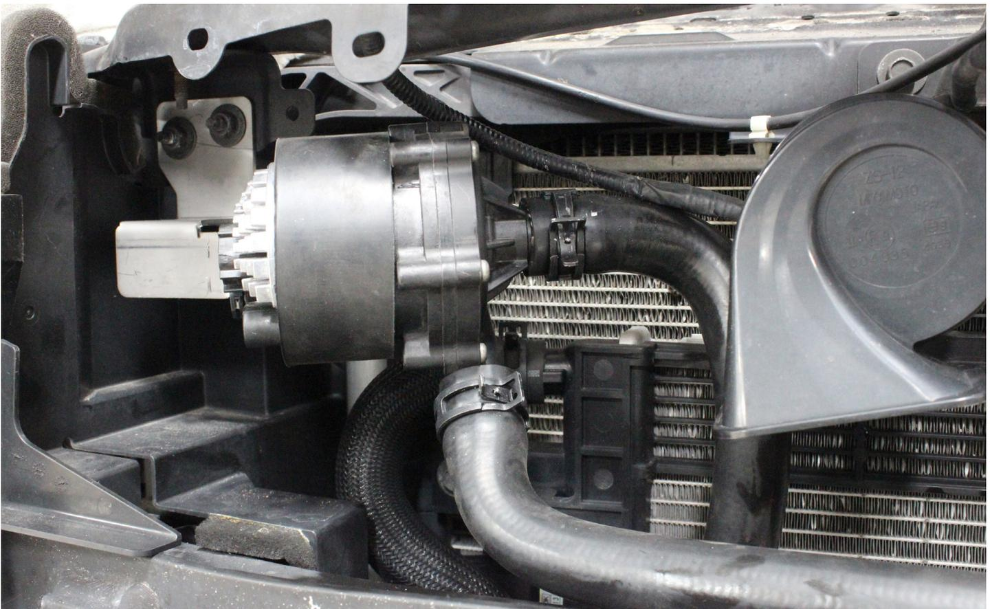
**20)** Lay the wiring harness out in the engine bay. Place the end of the harness with the relay, fuse, and ring terminals by the front right strut tower. Take care that the exposed metal on the harness does not short out the battery terminals. Feed the other end of the harness with the blue and grey pump connectors through the circled hole.
