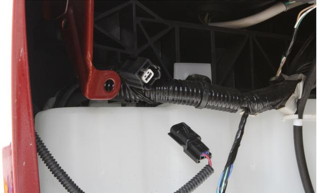
**7)** Inside the right-side wheel well just behind the bumper, locate and disconnect the two connectors for the parking sensors and front camera (if equipped).
