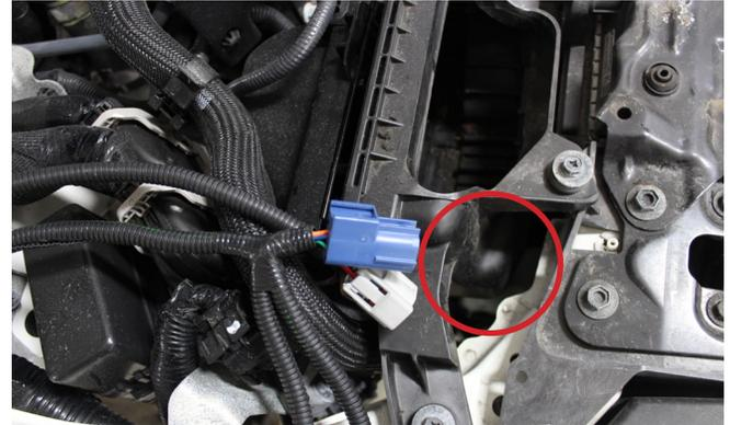
**21)** Route the harness down along the existing coolant line as shown. Disconnect the green OEM pump connector.
