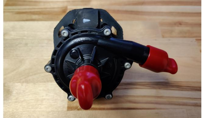
**16)** Remove the two nuts indicated and mount the pump. Tighten the two nuts back on to the studs.
