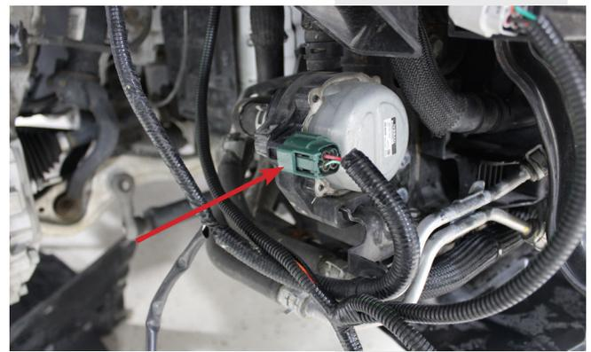
**22)** Plug the blue connector from the new harness into the green factory pump harness connector. Plug the shorter grey connector from the new harness into the factory pump.
