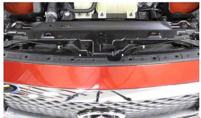
**12)** Carefully remove the front bumper. A second person is recommended for help. Make sure to pull the areas of the front bumper that meet the fender away from the headlights when removing. Masking tape is also highly recommended to protect any edges, panels, and headlights from being scratched during removal.
