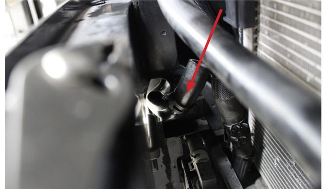
**19)** Attach hoses to the pump and secure with hose clamps as shown. The other end of the hose from the prior step will attach to the pump inlet (axial with the pump body). Ensure that the hoses are oriented such that they are not touching the heat exchanger or the crash beam. It is okay if the hoses lightly touch each other. The pump can also be adjusted within the rubber mounting grommet for alignment of the hoses.
