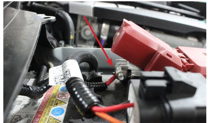
**30)** Undo the front battery tie down nut. Hold on to the hook as the nut is removed to prevent it from dropping down. Place the relay onto the tie down stud and reattach the nut. Place the mounting hole of the fuse holder over the stud. The hole is slightly undersized on the fuse holder so some pressure will be required.
