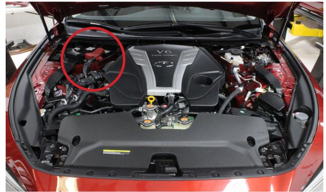
2) Remove the engine bay trim panels that run along the front fenders. These can be difficult to remove. Start at either end, pull straight upwards releasing the clips underneath. While pulling upwards, wiggle the panel around to try and release the clips. Plastic panel trim tools can also be used to get under the panel to pry upwards as well.
