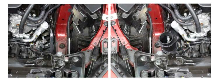
27. Place the left side (Driver) bracket into the rubber grommet on the frame rail. The top of the support bracket will sit just under the MAF housing mounting ear. Clock the silicone coupler and MAF housing so that the bracket perfectly aligns with the mounting ear. At this point, tighten the #32 hose clamp on the turbo inlet locking the
