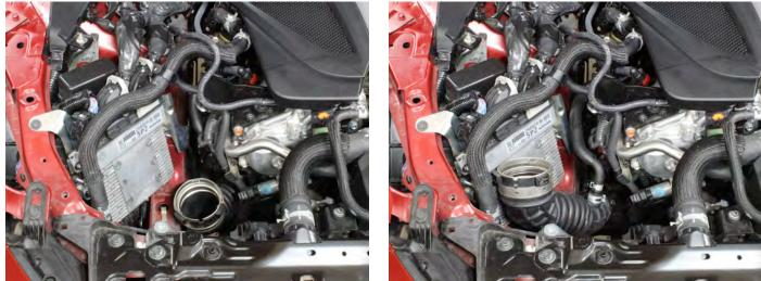
08. Disconnect the PCV hose from the OEM coupler. Only disconnect the small clamp at this time. Completely remove the OEM coupler.
