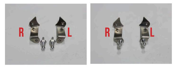
17. Place the right side (Passenger) bracket into the rubber grommet that was moved in step #9 as shown. The top of the support bracket will sit just under the MAF housing mounting ear. Clock the silicone coupler and MAF housing so that the bracket perfectly aligns with the mounting ear. At this point, tighten the #32 hose clamp on the turbo inlet locking the coupler in place.
