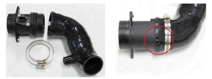
13. Once the silicone is installed on the MAF housing, tighten the #48 hose clamp as shown in the first picture below. The worm gear will align on the side of the MAF housing with the Pem nut. Loosely install the #32 hose clamp on the smaller end in the orientation shown.
