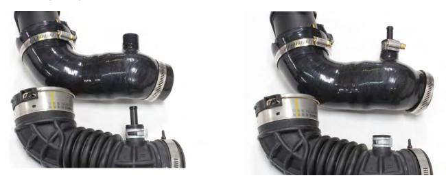
15. Install the silicone coupler in the car. First attach the PCV vent hose using the smaller OEM clamp. Then fully install the coupler onto the turbo inlet. Do not tighten the hose clamp yet.
