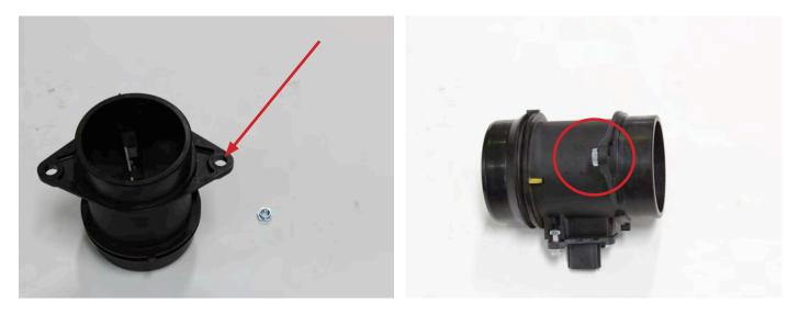
TECH NOTES: Pem nuts are often referred to as clinch style captive nuts. They press into a drilled or punched hole with an arbor press or similar pressure tool. In this case, as we're installing it into a plastic material, a pair of pliers will do the trick. Below is a close up of the Pem nut supplied. You can see the knurled area that is slightly tapered. This will lock the nut in place after it is pressed into the MAF housing.
