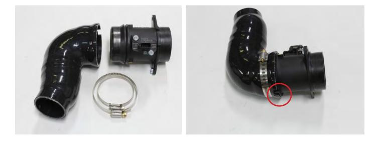
25. Once the silicone is installed on the MAF housing, tighten the #48 hose clamp as shown in the first picture below. The worm gear will align on the side of the MAF housing with the Pem nut. Loosely install the #32 hose clamp on the smaller end in the orientation shown.
