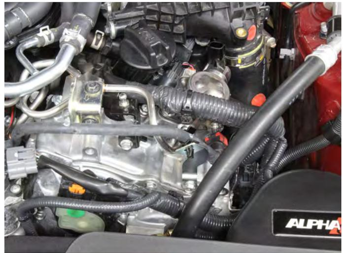
04. Make sure fuel pressure has been relieved as was explained in the first section of the instructions, and the engine is cool. Place a rag under the inlet and outlet fitting on the HPFP to catch any fuel left over in the lines. Start by releasing the red lock tab on the low side inlet fitting. Make sure not to force the red lock tab off as it could break. Carefully spread the two tabs at the top outwards and slide the lock tab downwards. Disconnect the fitting from the HPFP.
