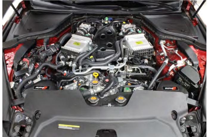
02. The HPFP is located on the left side of the engine (Driver's Side), just in front of the intercooler. First start by removing the bracket in front the pump. It is held in place by two 12mm bolts and holds three main harness clips plus one fuel line holder. Disconnect the harness clips and fuel line from its holder, remove the bracket.
