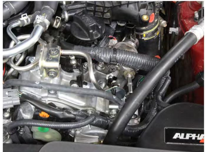
05. Next disconnect the high side line by using a 19mm open end wrench.
