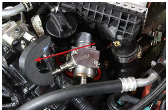
13. Once everything is lined up properly, install the two supplied M8 allen bolts. Make sure to tighten the bolts in steps the same way as was done during removal. Tighten the allen bolts to 22 ft lbs (29.5 N.m). Once the HPFP is torqued into place, tighten the high pressure fuel line coupler. Tighten the coupler nut to 27 ft lbs (36 N.m). Last, unbolt and re-tighten the high pressure line support bracket to take any unwanted stress off the line after the HPFP and fittings are tight.
