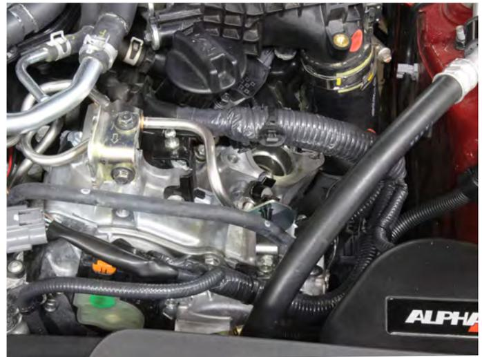
07. Make sure the surface of the cylinder head flange is clean. The OEM HPFP seals internally with an O-ring and the new Red Alpha HPFP seals on the surface of the flange with an O-ring installed in the base plate of the HPFP.
