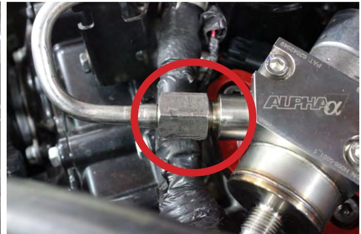
14. On the RA338 HPFP, reconnect the low pressure line and slide the red lock into place. A little silicone spray is recommended on the fitting to prevent damage to fitting O-rings. There is a support bracket that can be removed since the low side line location changes with the HPFP.
