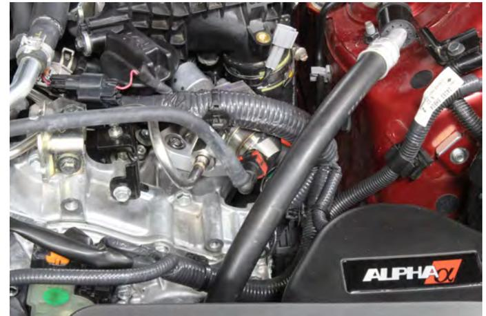
15. On the RA405 HPFP, the inlet fitting is a -6AN male fitting. The OEM plastic feed hose does not have the correct fittings. There are 3 options listed below for a low pressure feed hose...
