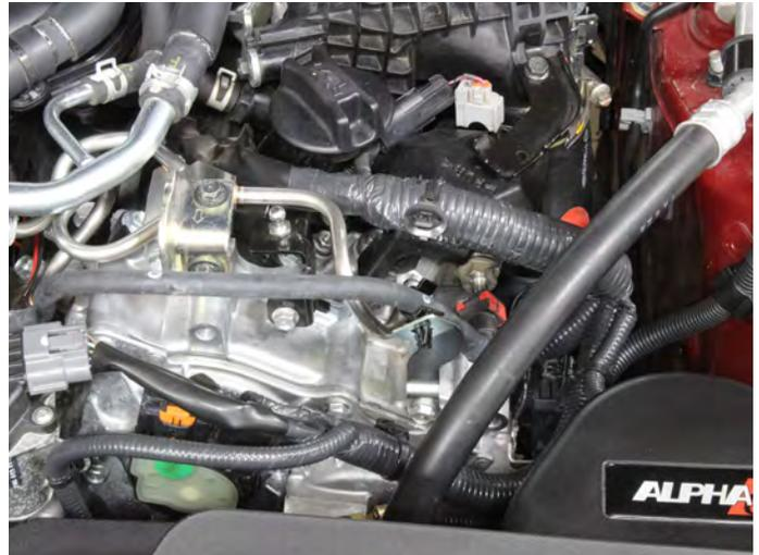
03. If equipped, remove the 10mm bolt and bracket bolted to the intercooler holding the sound deadening cover for the HPFP. Disconnect the connector at the HPFP and remove the cover.
