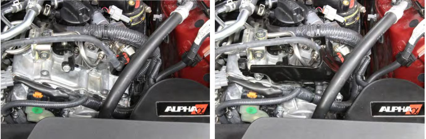
17. Double check all your connections. Reinstall the #52 (15A) fuse removed in the pressure relieving section. Prime and start the engine. Check all lines and fittings for leaks. Reinstall the engine cover once complete.
