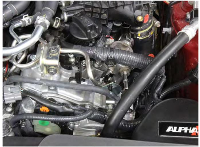
06. Loosen but do not remove the two 10mm bolts on the bracket supporting the high pressure line. Unbolt the HPFP but do so in steps loosening the bolts one turn at a time. You must do this due to the possibility of cam shaft lobe being at the top and the HPFP being under the load from its return spring. Remove the HPFP once fully disconnected.
