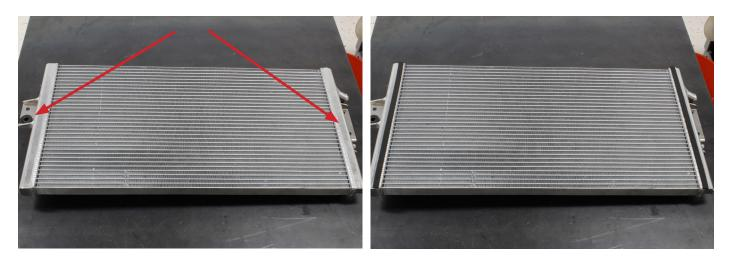
**31.** Carefully install the Infiniti Red Alpha heat exchanger in the car. Use the factory bolts and mount the heat exchanger loosely.
