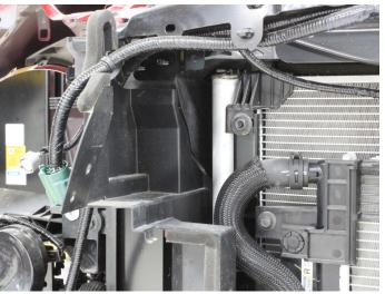
**22.** Remove the plastic air duct.
