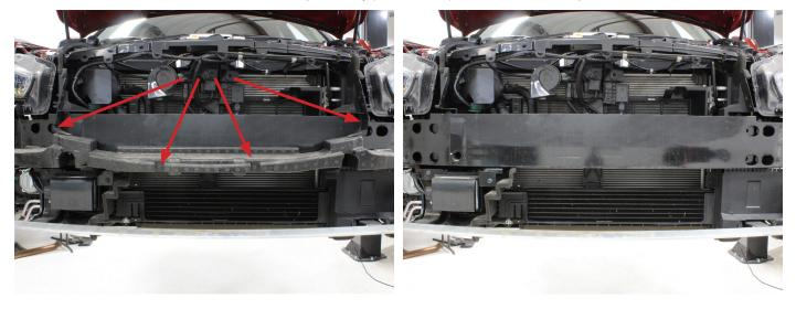
**14.** For the Q50 and Q60 if equipped, disconnect and remove the ICC (Radar Sensor) harness. The Q50 sensor is located in the lower right corner of the crash beam (shown). The Q60 is located on the top center of the crash beam.
