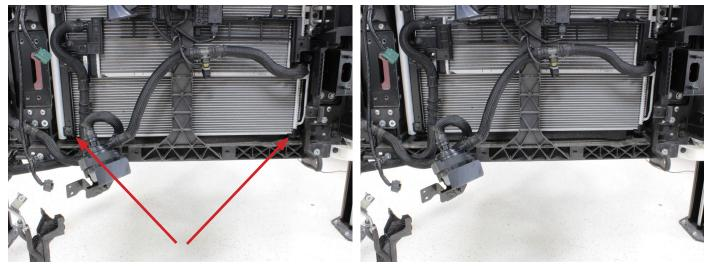
**27.** Disconnect the inlet and outlet hose on the factory heat exchanger. Make sure to have a drain pan under the disconnection point to collect coolant that still remains in the system.
