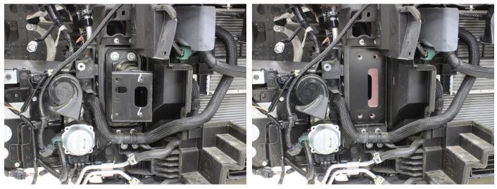
19. If equipped with an engine oil cooler, remove any plastic panels covering it.
