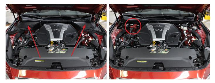
**02.** Remove the engine bay trim panels that run along the front fenders. These can be difficult to remove. Start at either end, pull straight upwards releasing the clips underneath. While pulling upwards, wiggle the panel around to try and release the clips. Plastic panel trim tools can also be used to get under the panel to pry upwards as well.
