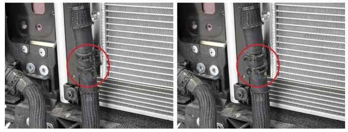
**35.** On the Q60 and Q50 Red Sport models, check the clearance of the secondary intercooler coolant pump inlet hose to the Infiniti Red Alpha heat exchanger. During reassembly, this area can be adjusted in two ways. First would be to bend the bracket slightly rotating the intercooler pump outwards and the hose away from the heat exchanger. The second would be to disconnect the pump inlet hose and using hose cutters, trim a small piece off making the hose slightly shorter.
