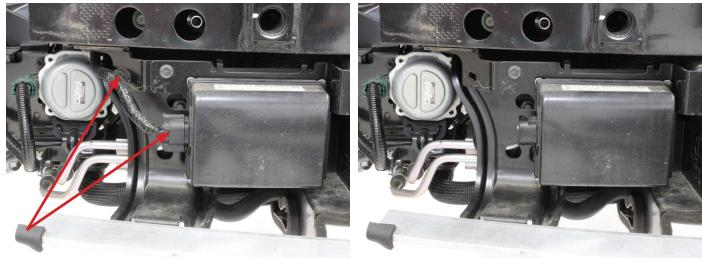
**15.** Remove the plastic panel that over laps the crash beam bracket.
