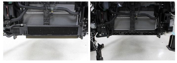
**21.** If you're Q60 or Q50 trim level is a Red Sport, you will need to unbolt the secondary water pump. Disconnect the electrical connector and unbolt the pump and bracket from the core support. You will not need to disconnect the hoses from the water pump. Allow the pump to hang.
