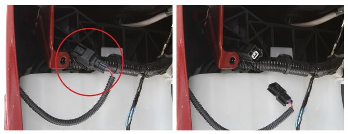
**07.** Inside the passanger side wheel well just behind the bumper, locate and disconnect the two connectors for the parking sensors and front camera.
