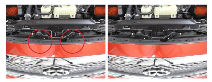
**12.** Carefully remove the front bumper. A second person is recommended for help. Make sure to pull the areas of the front bumper that meet the fender away from the headlights when removing. Painters tape is also highly recommended to protect any edges, panels, and headlights from being scratched during removal.
