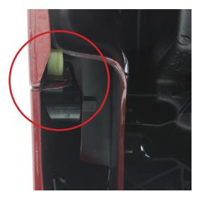
**10.** Just above the headlights where the top of the bumper and the fender meet, there is a bolt and retainer plate holding the two together. Remove the hardware shown.
