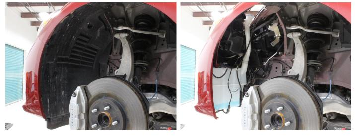
06. Disconnect the front LED running light harnesses on both sides. The connectors are located just below the headlights.
