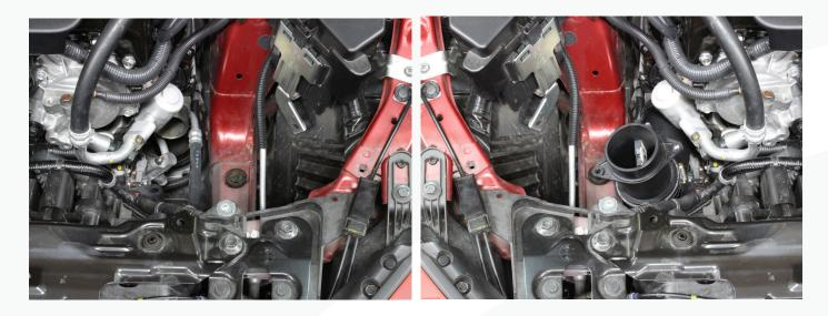
27. Place the left side (Driver) bracket into the rubber grommet on the frame rail. The top of the support bracket will sit just under the MAF housing mounting ear. Clock the silicone coupler and MAF housing so that the bracket perfectly aligns with the mounting ear. At this point, tighten the #32 hose clamp on the turbo inlet locking the coupler in place.
