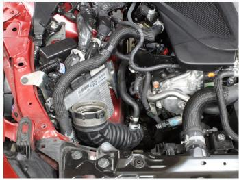
08. Disconnect the PCV hose from the OEM coupler. Only disconnect the small clamp at this time. Completely remove the OEM coupler.
