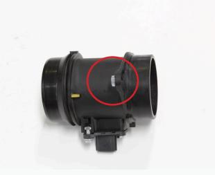
TECH NOTES: Pem nuts are often referred to as clinch style captive nuts. They press into a drilled or punched hole with an arbor press or similar pressure tool. In this case, as we're installing it into a plastic material, a pair of pliers will do the trick. Below is a close up of the Pem nut supplied. You can see the knurled area that is slightly tapered. This will lock the nut in place after it is pressed into the MAF housing.
