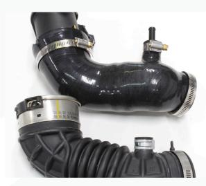
15. Install the silicone coupler in the car. First attach the PCV vent hose using the smaller OEM clamp. Then fully install the coupler onto the turbo inlet. Do not tighten the hose clamp yet.
