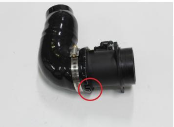
25. Once the silicone is installed on the MAF housing, tighten the #48 hose clamp as shown in the first picture below. The worm gear will align on the side of the MAF housing with the Pem nut. Loosely install the #32 hose clamp on the smaller end in the orientation shown.
