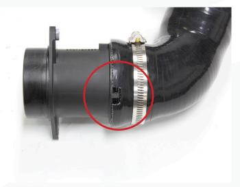
13. Once the silicone is installed on the MAF housing, tighten the #48 hose clamp as shown in the first picture below. The worm gear will align on the side of the MAF housing with the Pem nut. Loosely install the #32 hose clamp on the smaller end in the orientation shown.
