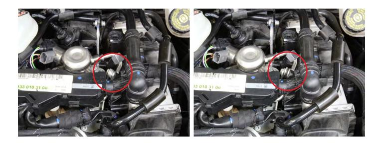
**08.** Remove the 2 screws securing the hardline support bracket. Then remove the bracket from the vehicle. This bracket will not be reused.
