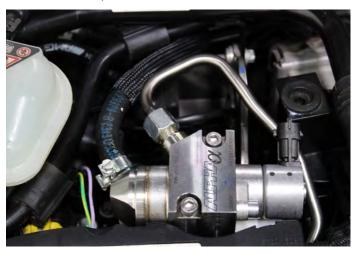
15. Install the silicone coupler in the car. First attach the PCV vent hose using the smaller OEM clamp. Then fully install the coupler onto the turbo inlet. Do not tighten the hose clamp yet.
