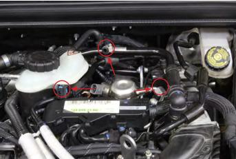
**04.** Remove the plastic engine cover mounting stud.
