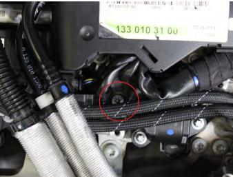
**06.** Lift up on the main engine wire harness to gain access to the union nut on the high pressure hardline where it connects the fuel rail. There is a stud the plastic harness loom clips into between the intercooler and cylinder head. Move the harness towards the intercooler to release the harness off this stud. You may be required to use a flat head to pry it off the stud in certain cases. Disconnect the fuel line from the rail.
