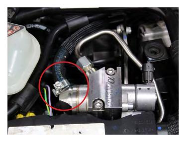
14. Locate the supplied HPFP wire harness adaptor. Install and route the harness as shown below
