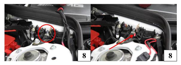
**9)** There is a fuse holder and a momentary switch. Make sure the 25 amp fuse is installed. The momentary switch when pressed will turn on both pumps. This switch will aid in bleeding the system. You may mount the fuse holder and switch anywhere you like. We have supplied a M6 bolt and nut. We chose to mount the fuse holder as shown in the picture to the battery cable cover.
