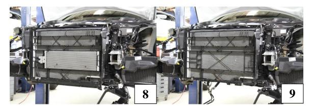
**10**) Drain the A/C system. The A/C condenser will need to be removed.
