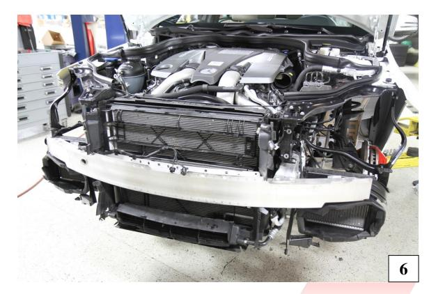
7) Remove the front crash bar. **Caution**, there are two SRS sensors on the back of the bar. Take care in disconnecting the connectors and removing the bar.
