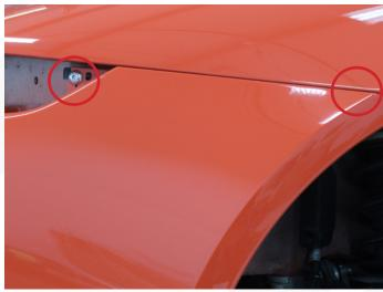
09. Remove the two T30 Torx Screws from the inside of the wheel well area on each side.
