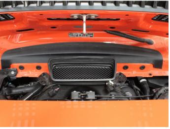
**15.** Remove the 10mm bolt holding the oil fill cap assembly in place. Pull the plate off the wing assembly and set it off to the side leaving the cap on.
