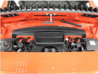
**03.** Disconnect and remove both the fans. Take care when pulling the fans off the mounting ball and grommets so not to break a tab off.
