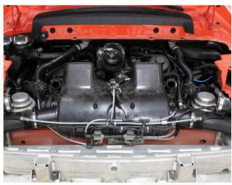
21. Unclip the solenoid at the top of air box. Pull the lines off the retainers on the top of the air box as well and pull them towards the rear of the car. There is only one of the plastic lines you need to disconnect. It is the line shown on the right side of the air box where the clear tube transitions into a black tube. Everything else can be left connected.
