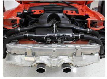
19. Remove the top air box inlet duct. Carefully pry the ball mount out of the grommets holding the duct in place.
