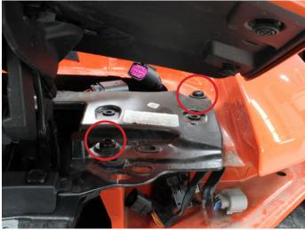
18. With the wing assembly removed, remove the two intercooler inlet ducts.
