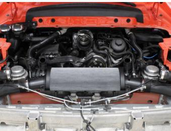
23. Reinstall the air box lid in the reverse order of removal. When reconnecting the solenoid and hoses, make sure to use the supplied zip on the hose attached to the bottom of the right side air filter outlet as shown. This will help keep the line attached with heat and vibration present in this location.
