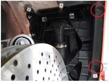
**10.** Unclip the two connectors behind the right rear taillight area and disconnect them. The harness will come with the bumper when removed.
