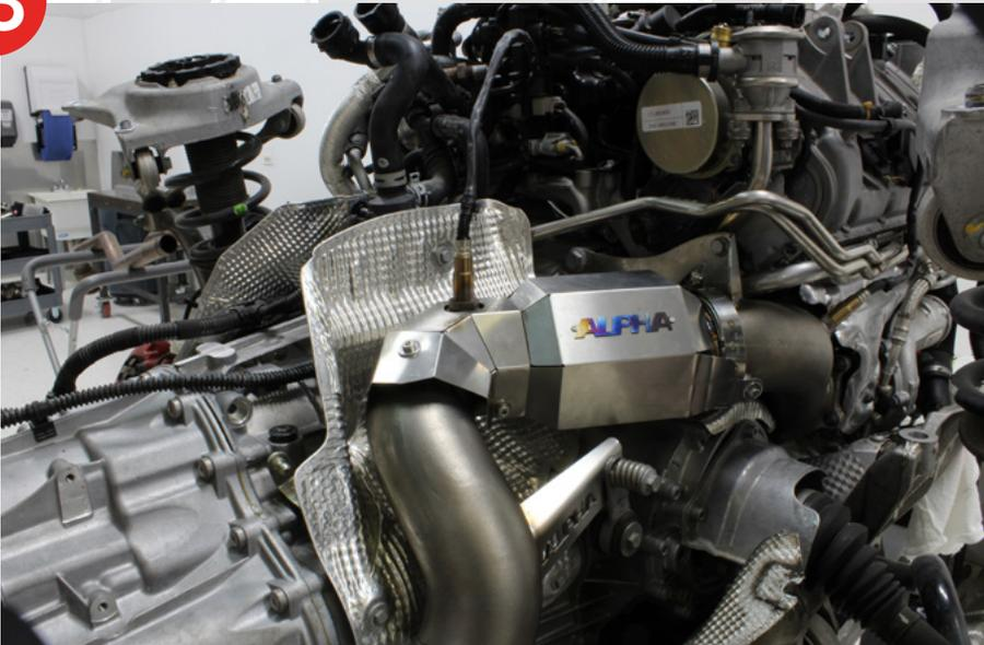
**14.** Remove the studs from the right side midpipe. This can be done on a press or using heat and hammering them out. Take care not to damage the flange. New studs for the downpipe have already been installed. Having the studs installed in the downpipe allows easier removal of the midpipes. New midpipe to downpipe nuts and gasket have been included.
