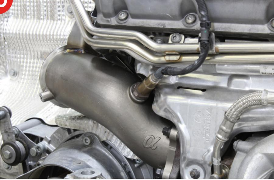
11. Install the second half of the downpipe using the new supplied V-band clamp and reusing the spring bolt. Clock the V-band bolt as shown below. The stud should be facing upwards towards the inside of the engine. Use the supplied M8 nut on the back side of the spring bolt.
