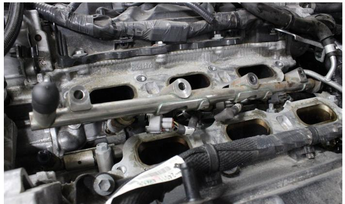
21. Disconnect the driver side fuel rail connector and remove the bolts holding the fuel rail. Remove the fuel rail.
