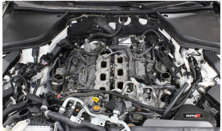
**NOTE:** If you have not already, clean up any debris in or around the valley of the engine. Any contaminants in the fuel system can lead to injector failure. Also, it is a good idea to use paper towels to plug the intake ports to keep debris from falling in while the manifold is off.
