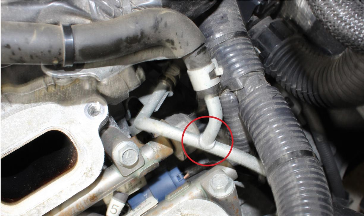
20. Due to the design of the fuel rails, the passenger rail needs to be removed first. Remove the two nuts and two bolts holding the passenger side fuel rail to the cylinder head. Work the rail free and remove it as shown below.
