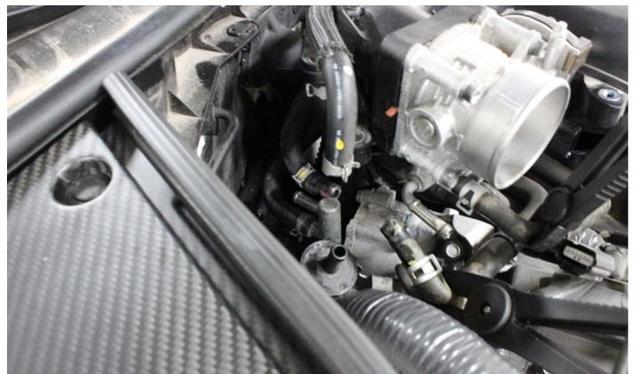
13. Using a long flat blade screwdriver, release the clip and pull the hose off the bracket.
