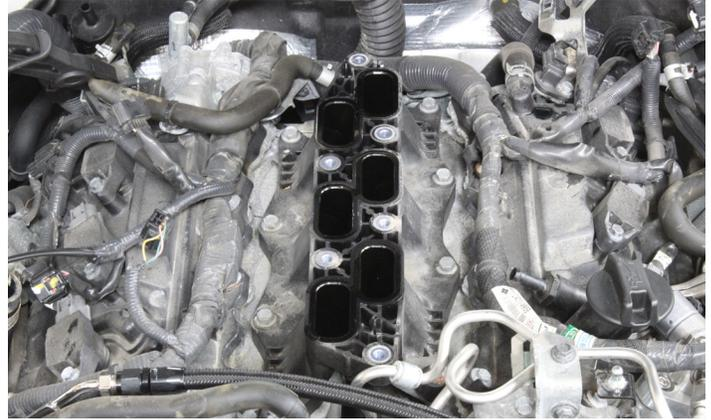
16. Remove eight lower intake bolts to remove the lower intake.
