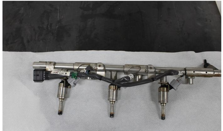
23. Replace each injector by disconnecting the connector and removing from the rail. Apply a small amount of O-ring safe grease to the new o-rings. Ensure that none of the grease ends up in the inlet of the injectors.
