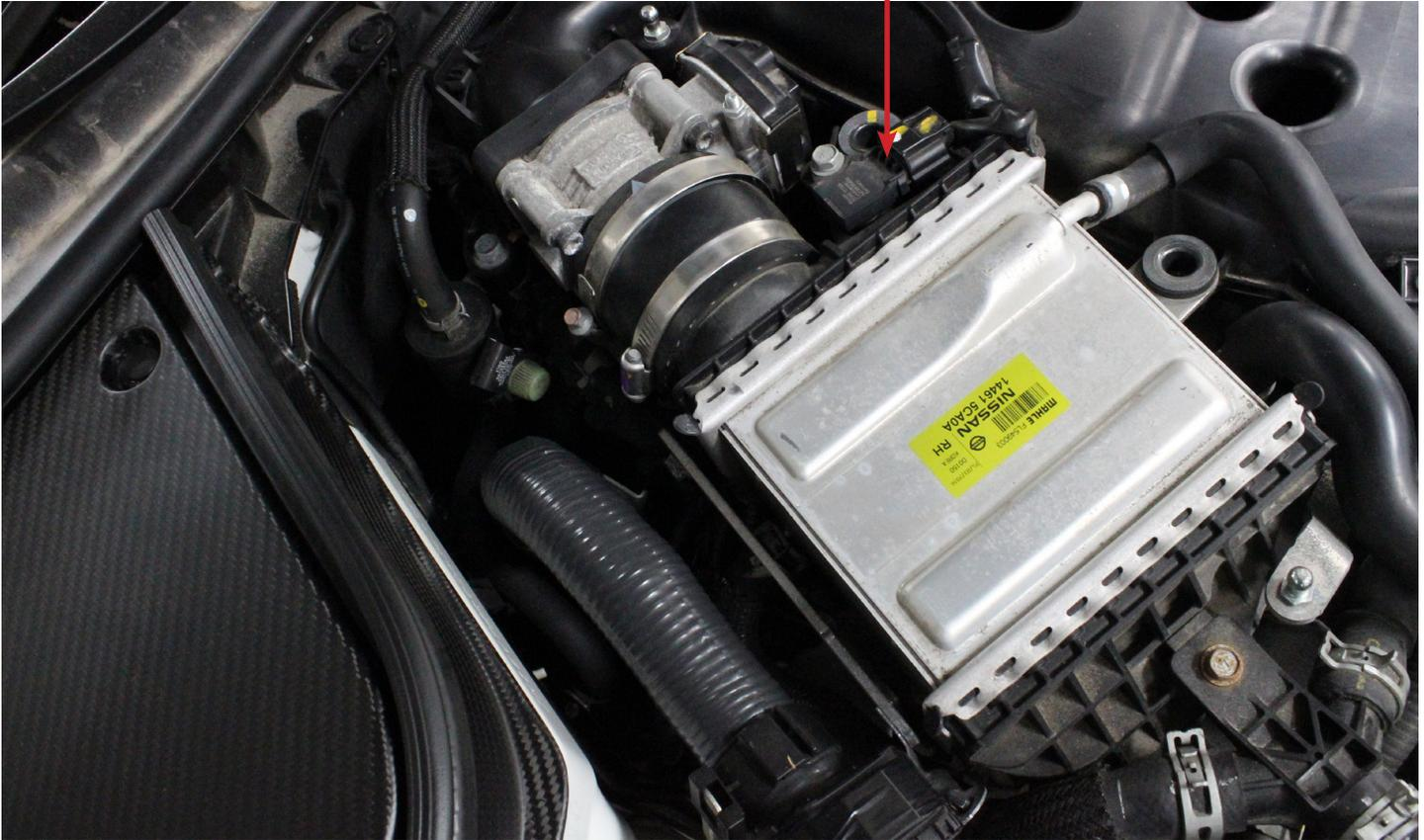
4. Disconnect the hose and remove the bolt holding the bracket.
