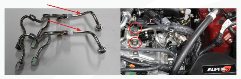
12) On the STAGE 3 HPFP, we have supplied a high pressure line template. The template is 3D printed and aids in the bending of the line properly. This tool is not used to bend the line but to check it being bent correctly. The plastic template slides over
