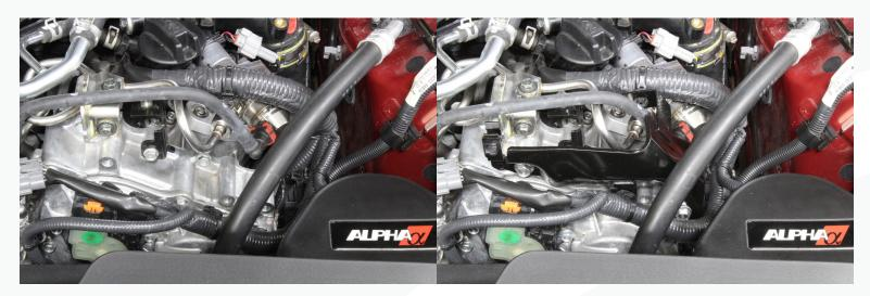
17) Double check all your connections. Reinstall the #52 (15A) fuse removed in the pressure relieaving section. Prime and start the engine. Check all lines and fittings for leaks. Reinstall the engine cover once complete.
