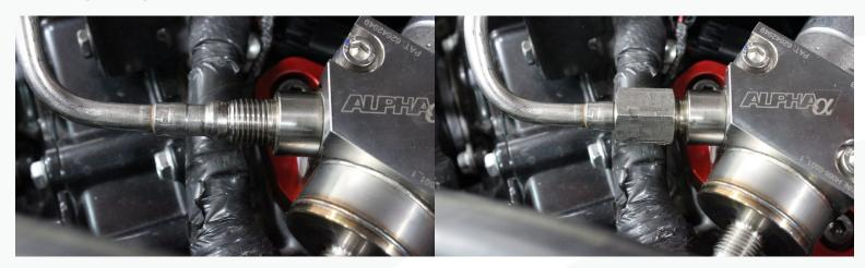
14) On the STAGE 1 HPFP, reconnect the low pressure line and slide the red lock into place. A little silicone spray is recommended on the fitting to prevent damage to fitting O-rings. There is a support bracket that can be removed since the low side line location changes with the HPFP.
