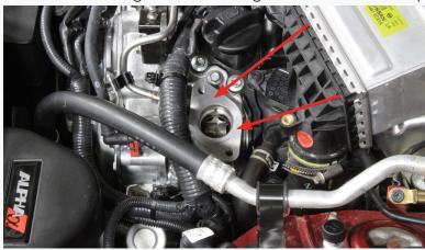
**Note**: The next step will require the help of an additional person. You will be required to make sure the fuel pump bucket that rides on the cam is at its lowest position. Due to the heavy spring installed on the HPFP for high RPM use, damage to the cylinder head threads for the HPFP could happen if this is not done. Do not draw the pump down using the bolts if the cam lobe is not at its lowest point!
