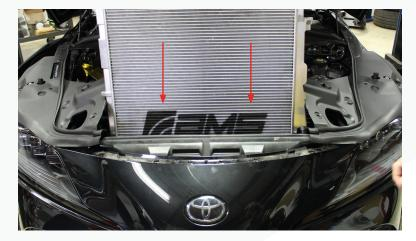
9. Once the AMS heat exchanger has been fitted, the rest of the installation is a reverse of the disassembly process. Make sure the heat exchanger fittings are properly clipped in place before installing any cover panels or refilling the system. All covers and hardware are installed back in their original locations.
