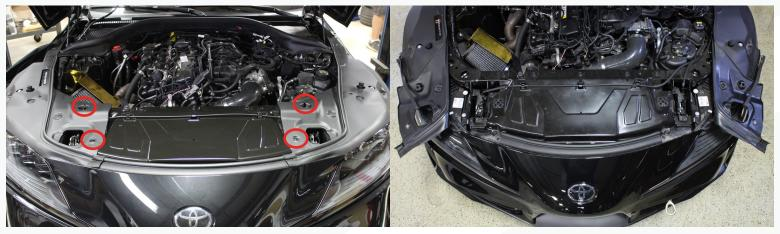
2. Remove the front hood seal and the six 10mm bolts underneath. Gently pull the nose piece of the bumper free of its mounting clips. With that out of the way, you can gain access to the 13mm cover panel bolts. Loosen the four front bolts and remove the rest. Unclip the hood release cable and the panel will slide backwards and then pull up.
