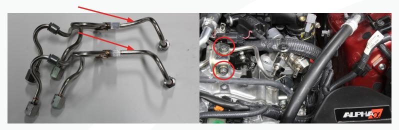
12) On the RA 405 HPFP, we have supplied a high pressure line template. The template is 3D printed and aids in the bending of the line properly. This tool is not used to bend the line but to check it being bent correctly. The plastic template slides over
