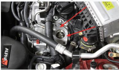
**Note**: The next step will require the help of an additional person. You will be required to make sure the fuel pump bucket that rides on the cam is at its lowest position. Due to the heavy spring installed on the Red Alpha HPFP for high RPM use, damage to the cylinder head threads for the HPFP could happen if this is not done. Do not draw the pump down using the bolts if the cam lobe is not at its lowest point!
