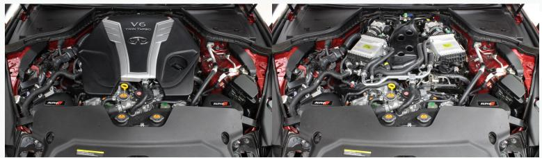
2) The HPFP is located on the left side of the engine (Driver's Side), just in front of the intercooler. First start by removing the bracket in front the pump. It is held in place by two 12mm bolts and holds three main harness clips plus one fuel line holder. Disconnect the harness clips and fuel line from its holder, remove the bracket.
