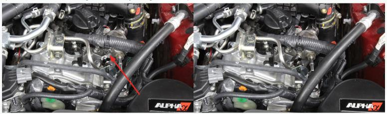
6)Loosen but do not remove the two 10mm bolts on the bracket supporting the high pressure line. Unbolt the HPFP but do so in steps loosening the bolts one turn at a time. You must do this due to the possibility of cam shaft lobe being at the top and the HPFP being under the load from its return spring. Remove the HPFP once fully disconnected.
