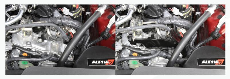
17) Double check all your connections. Reinstall the #52 (15A) fuse removed in the pressure relieaving section. Prime and start the engine. Check all lines and fittings for leaks. Reinstall the engine cover once complete.
