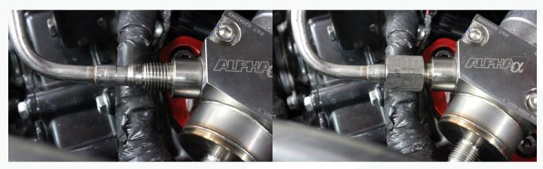
14) On the RA 338 HPFP, reconnect the low pressure line and slide the red lock into place. A little silicone spray is recommended on the fitting to prevent damage to fitting O-rings. There is a support bracket that can be removed since the low side line location changes with the HPFP.
