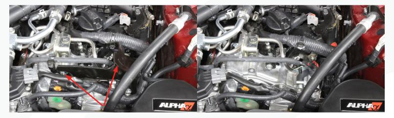
3) If equipped, remove the 10mm bolt and bracket bolted to the intercooler holding the sound deadening cover for the HPFP. Disconnect the connector at the HPFP and remove the cover.
