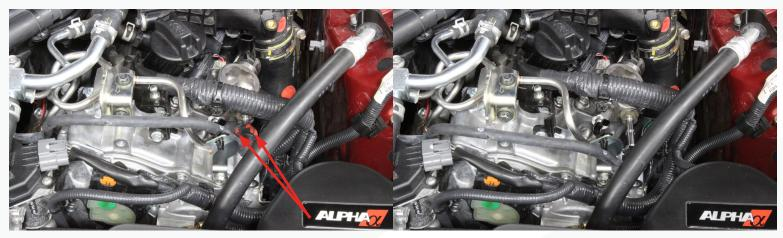
5) Next disconnect the high side line by using a 19mm open end wrench.
