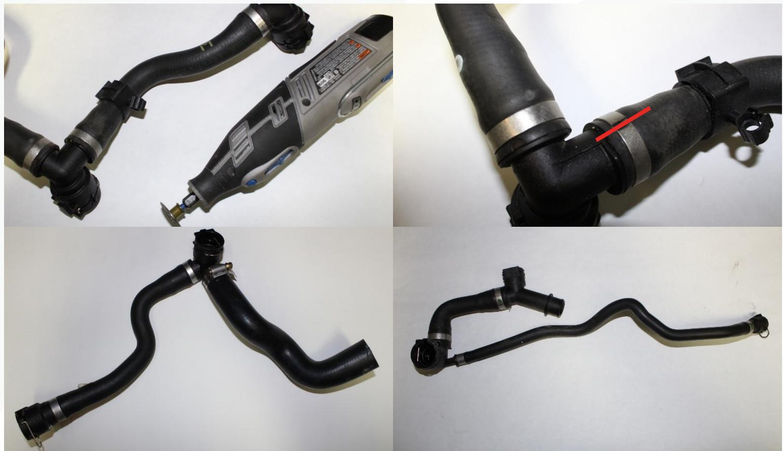
11. The longer hose will be installed on the intake manifold before being dropped into place. This will make the hoses easier to route and install in the engine bay. See pictures above for the correct orientation of this hose and make sure the hose clamp is tight.
