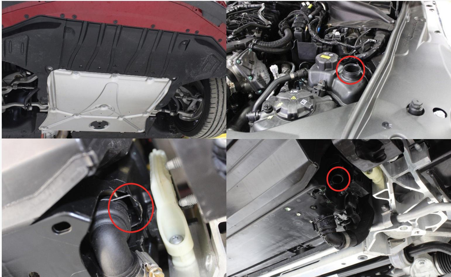
2. Remove the engine cover and charge pipe by removing the two bolts on the throttle body and metal retaining clip near the turbo. Stock charge pipe is shown, for the AMS charge pipe, loosen the worm gear clamps and remove the charge pipe.
