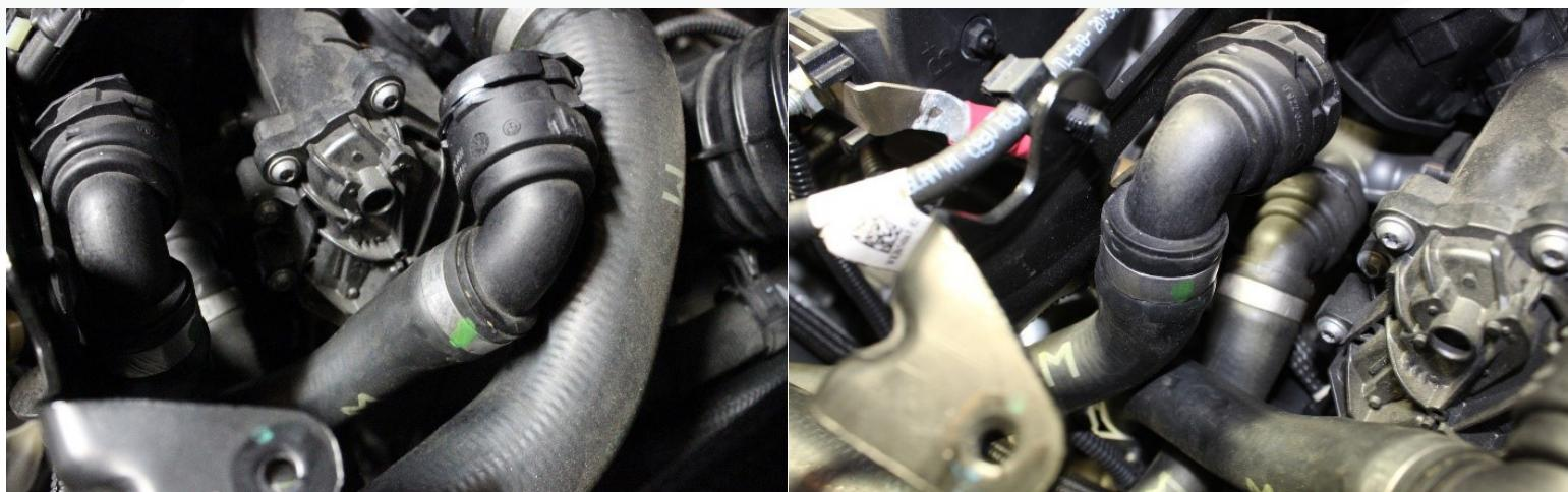
6. Once both fittings are removed, double check that all lines and connectors are removed from the manifold. Next, remove the seven 10mm bolts that mount the intake to the cylinder head. These are captured bolts and will not come all the way out of the intake manifold so do not force them. Then remove the two E-Torx head bolts on the outside support brackets for the manifold. Once these are removed, the intake can be lifted out of the engine bay.
