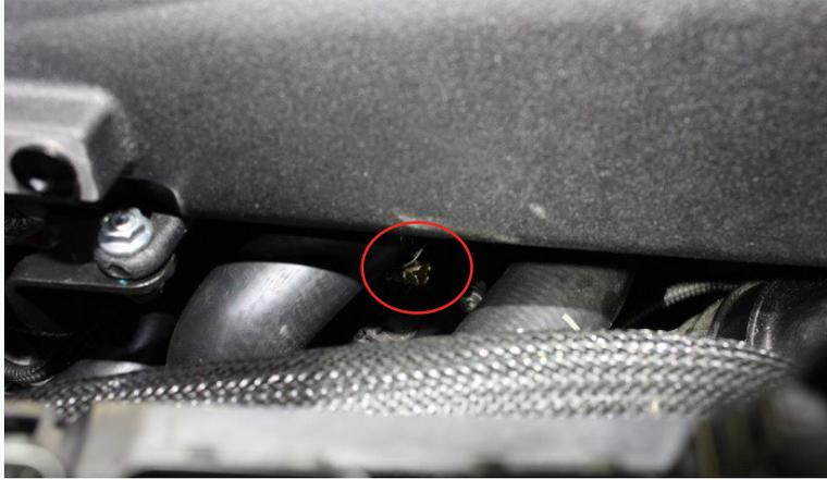
18. With the manifold in place, now assemble your fuel vapor feed hoses. Using the existing hoses cut off the hoses with a razorblade by carefully cutting a small incision where the hose meets the connector (pictured above), make sure not to cut too deep as you will damage the connector.
