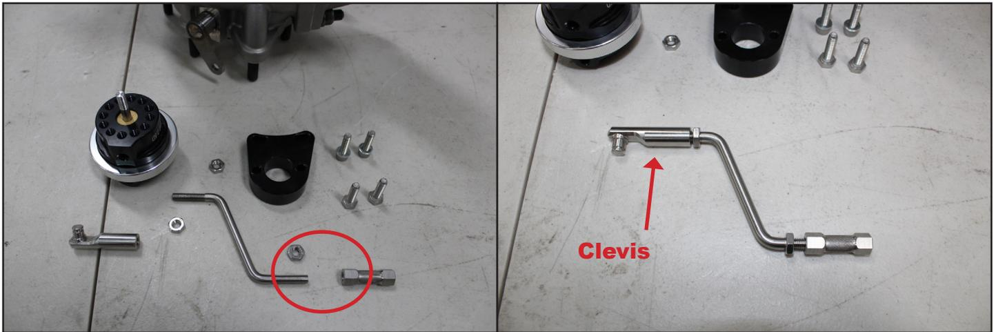
2. The remaining nut will go on the wastegate. Then install the rod assembly onto the wastegate. Be sure all the components are threaded on as far as you can but still loose.
