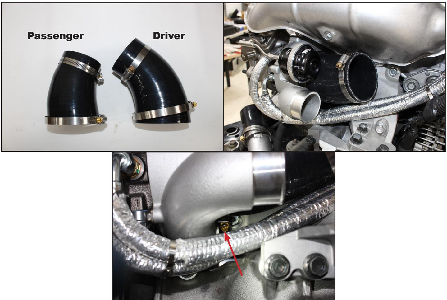
15. Locate the two charge pipe jumper silicones, two #32 clamps, and two #28 clamps. Install the longer jumper on the passenger turbo and reinstall the stock cast charge pipes. You will need to cut off the harness feature on the charge pipe to fit the intake pipe in the next step.
