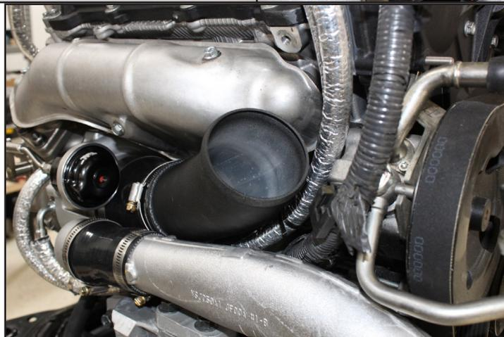
17. The last coupler needed on this side is the 3" straight coupler. This will connect to the intake system of your choice and can also be installed once the engine is in the car.
