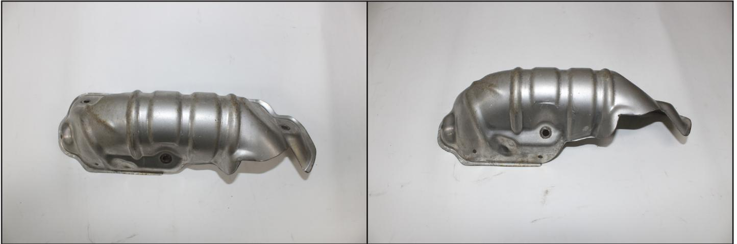
20. Using the provided bolts and one spacer, install the driver side heatshield. The longer bolt and spacer will be used in the location above the compressor cover as shown below. Place the spacer between the manifold and heatshield.
