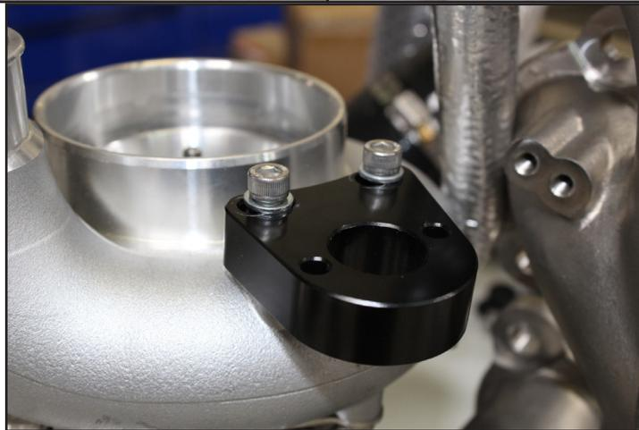
4. Place the assembly into the bracket on the turbo. Use the 7/8" long hex head bolt to attach the bracket to the wastegate. Use the threaded hole that is one hole over from the ports on the wastegate. Install the second bolt and tighten them both.
