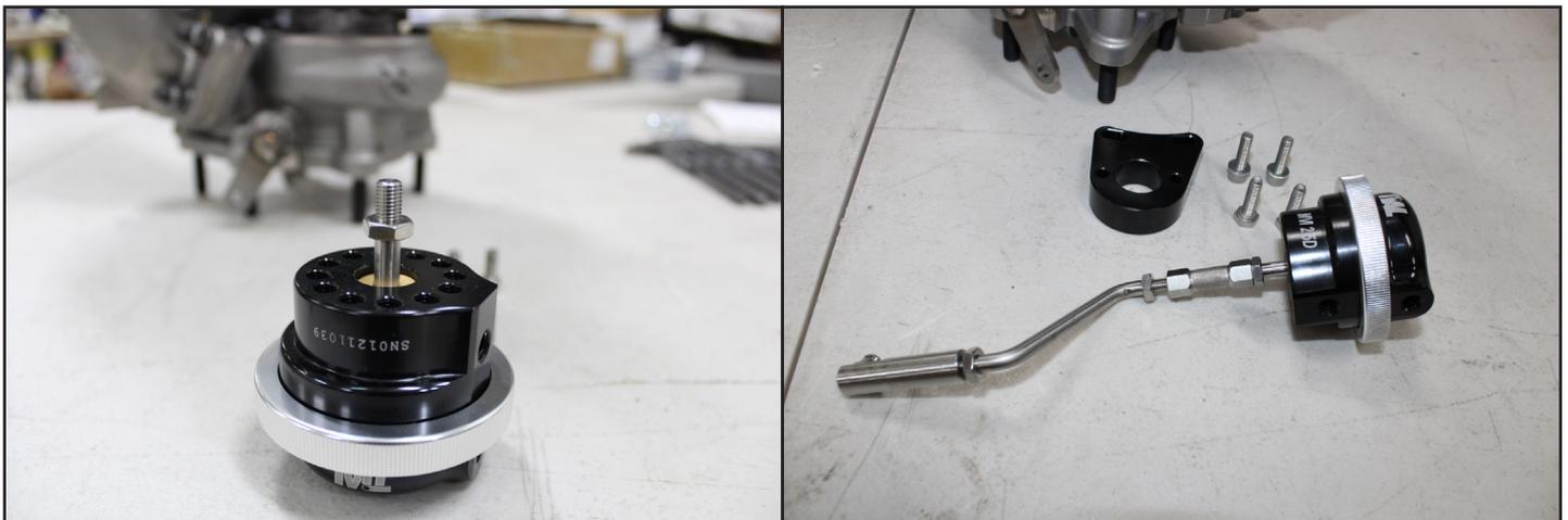
3. Locate the wastegate mounting hardware. Then locate the wastegate lever on the turbo assembly. LOOSLY install the bracket onto the compressor over with the two socket head bolts with washers.
