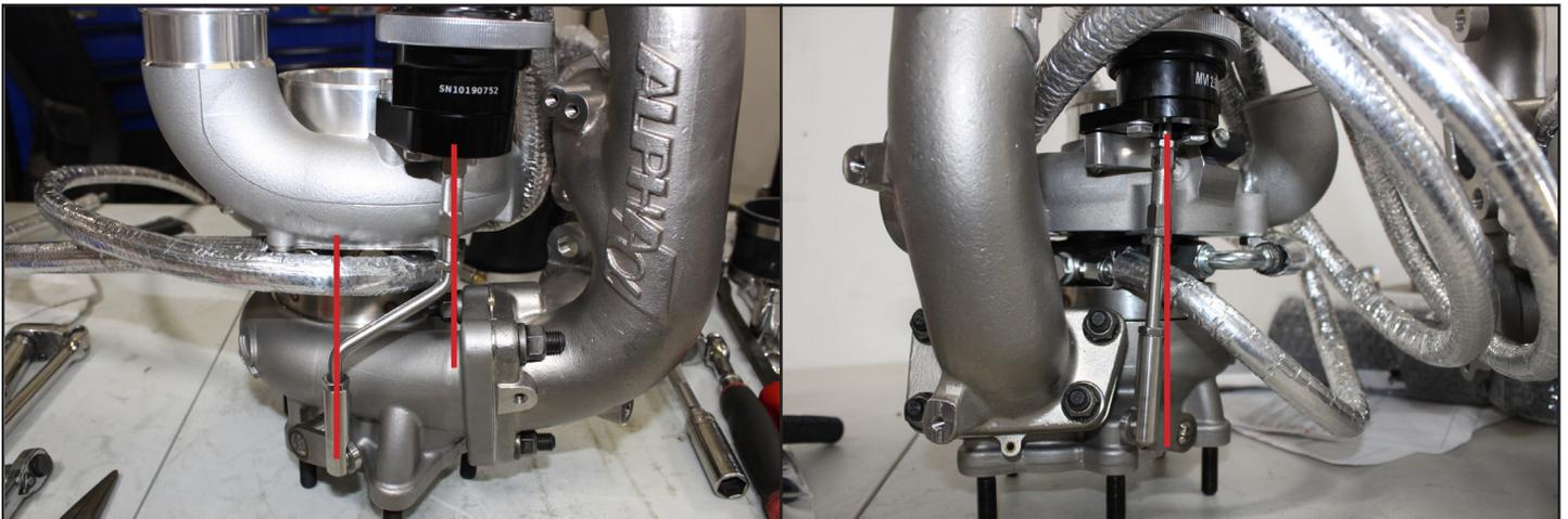
7. Once the rod is properly aligned. Tighten the two socket head bolts holding the bracket to the compressor cover.
