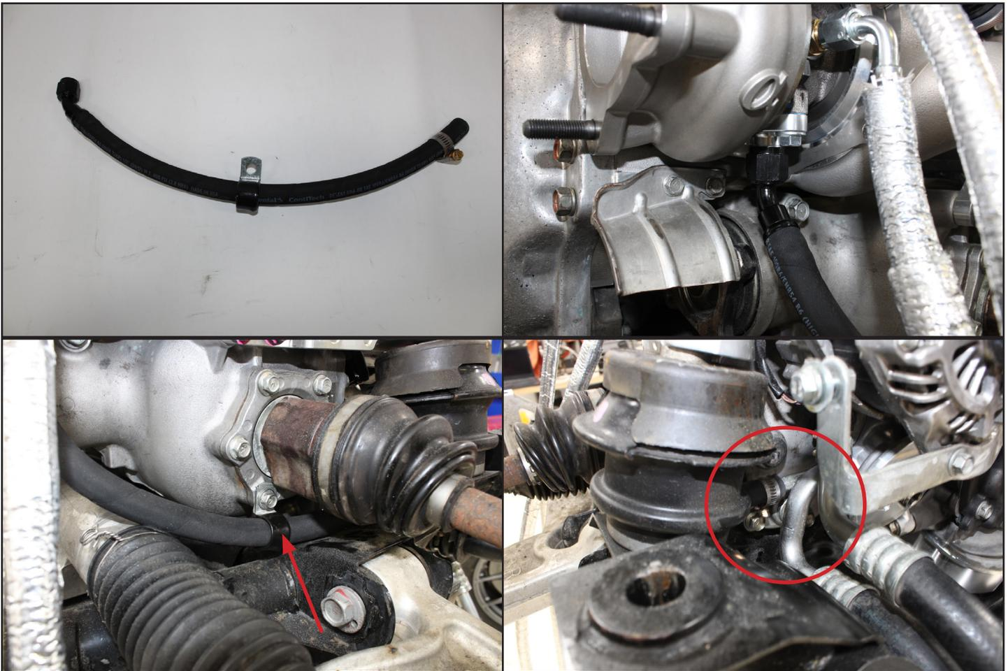
8. Mount the provided coolant hard pipe on the back of the engine on the crossover pipe. Reconnect the OEM hoses to the new Y pipe.
