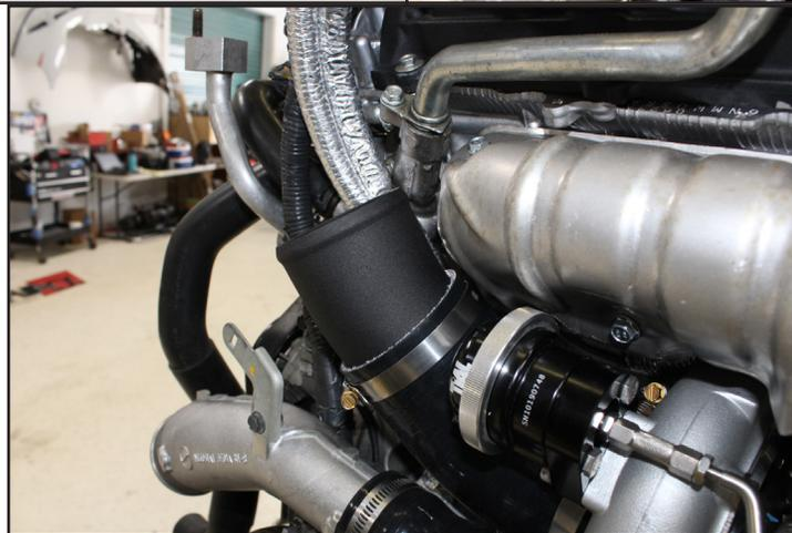
28. The last coupler connects to the intake system of choice and can be installed now or after the engine is in.
