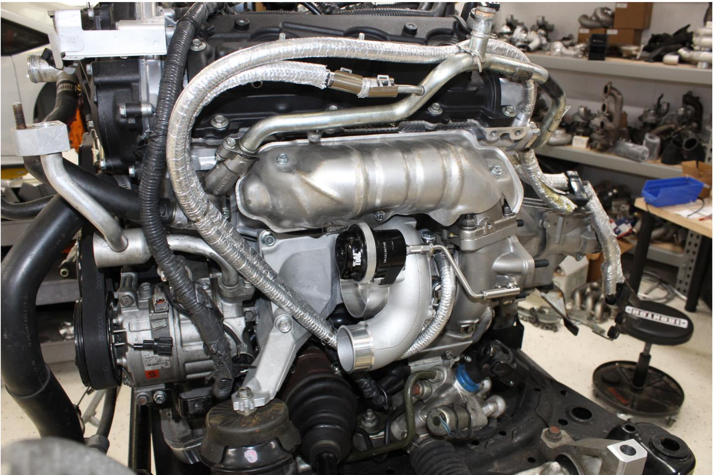
25. Using the remaining shorter charge pipe silicone and two clamps, reinstall the cast charge pipe.
