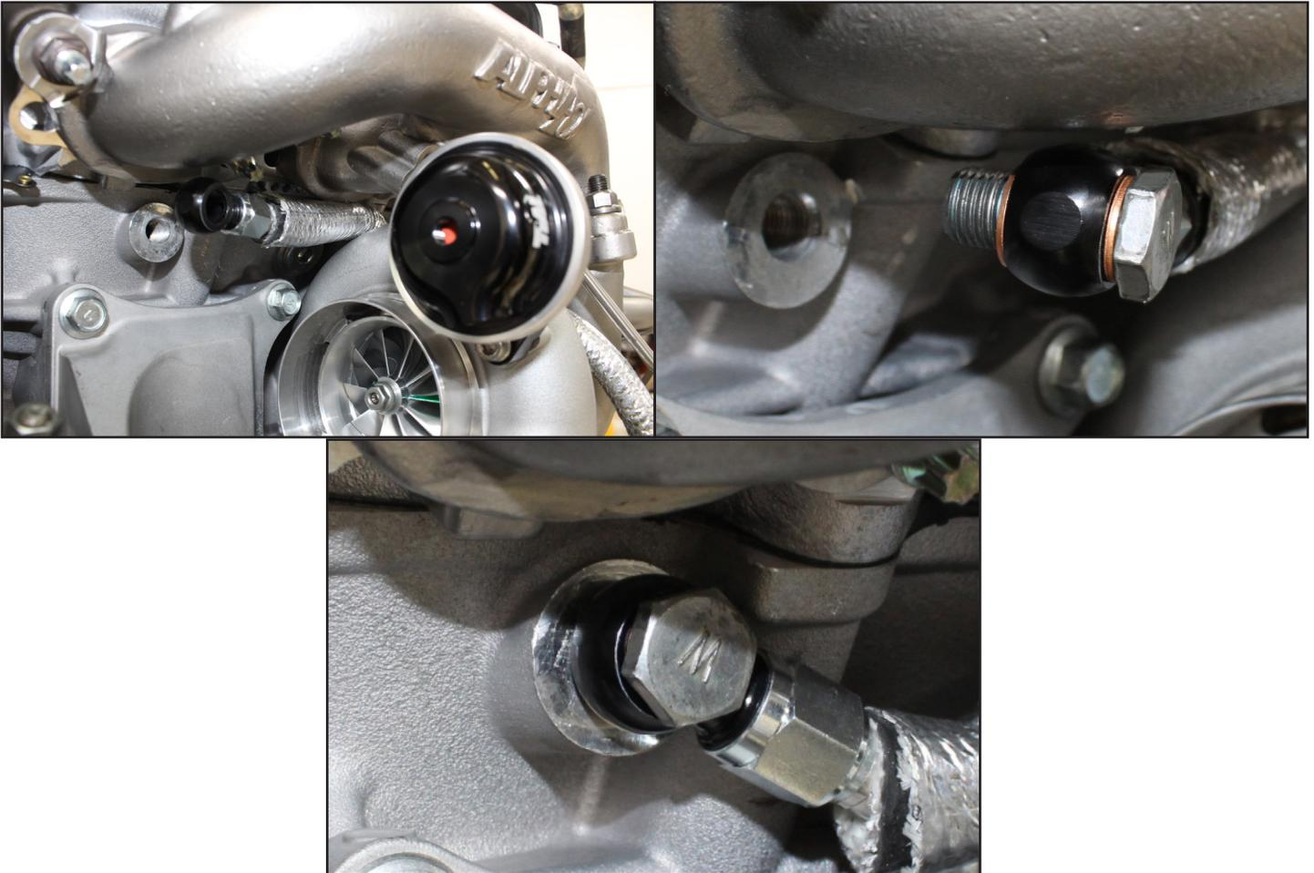
23. Route the oil feed and coolant line similar to the passenger side. Coolant line will hook to the OEM rubber line by the valve cover, and the oil line will route to the oil distribution block on the back of the motor.
