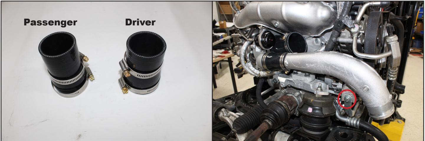
16. Find the two intake pipes, install the longer pipe on the passenger side with the bend side facing out. Try to clock the intake silicone and pipe tucked close to the engine for the most amount of clearance.
