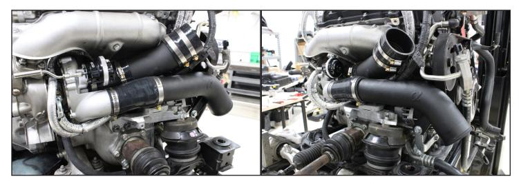
3. On the drivers side you will need the longer straight silicone and shorter cast charge pipe. Loosely install the silicone with two clamps.
