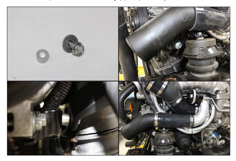
5. The charge piping kits includes silicone that routes from the cast compressor outlets to the inlet of the intercooler. If you already have an Alpha Intercooler setup, the 90-degree silicone will be changed. The old silicone is not a full 3" all the way through as the X kit silicone is.
