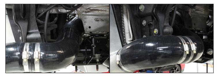
7. Locate the right-side compressor outlet kit silicone. Install the long S style silicone with the tight 45-degree downward bend on the cast compressor outlet pipe. Next install the supplied 3" jumper pipe. Last, install the 90-degree silicone with the longer leg on the intercooler. Leave all the hose clamps loose to adjust before tightening. Adjust as necessary, then finish tightening all the hose clamps starting from the cast outlet to the intercooler.
