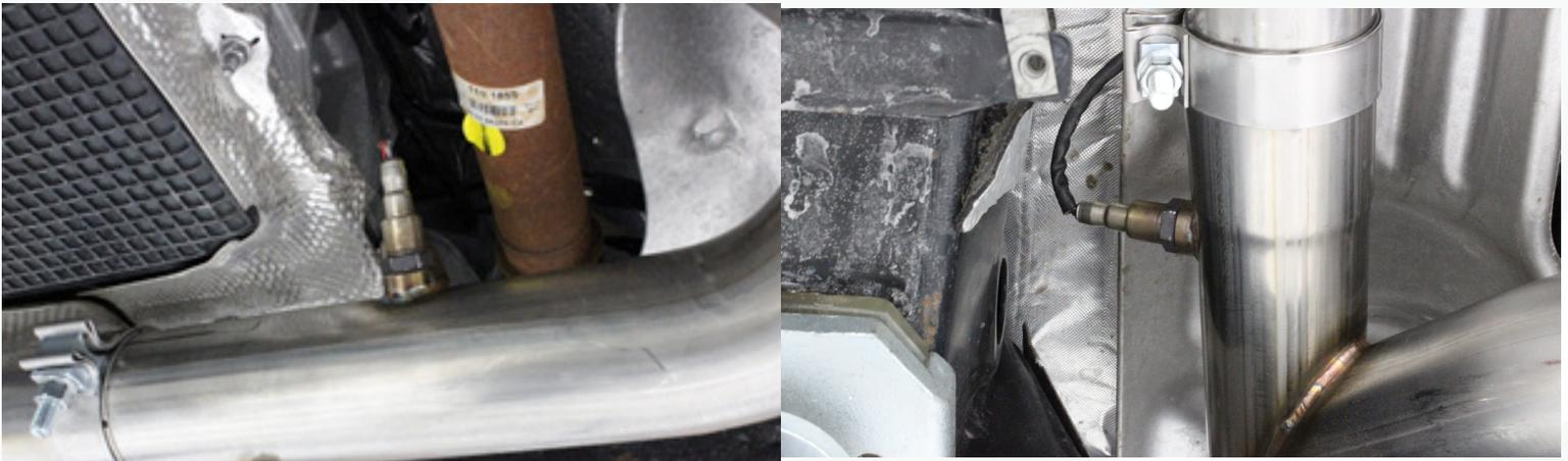
24) Re-assemble any parts that are left in reverse order of removal. Be sure to tie up any loose harnesses away from heat sources and rotation drivetrain parts.
