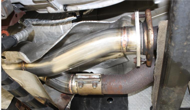
22) Reinstall the transmission mount and cross member. Once everything is installed and the downpipe is aligned, tighten the two-bolt flanges first starting with the connection at the turbo. You must be careful to tighten these flanges evenly. Failure to do so may result in exhaust leaks and/or damage to the ball seal and flange. Next, tighten the two-bolt flange to exhaust, followed by the band clamps.
