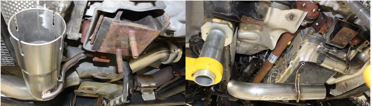
20) Mate the two ends of the driver side downpipe together and push them up into each other. The hanger will align into position in this step. Tighten the band clamp.
