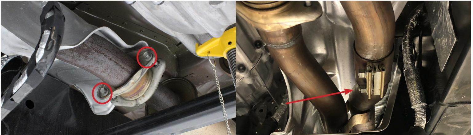
12) Disconnect both left and right side two-bolt flanges from the turbine outlet flanges. Save the nuts as they will be reused.
