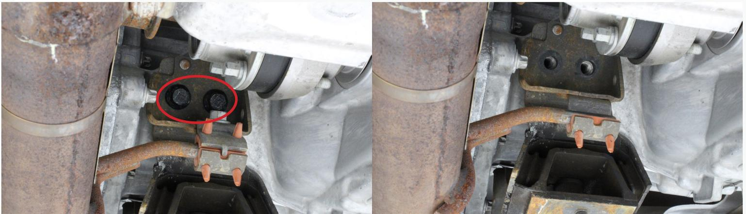
9) Remove the other two bolts from the transmission mount on the passenger side.
