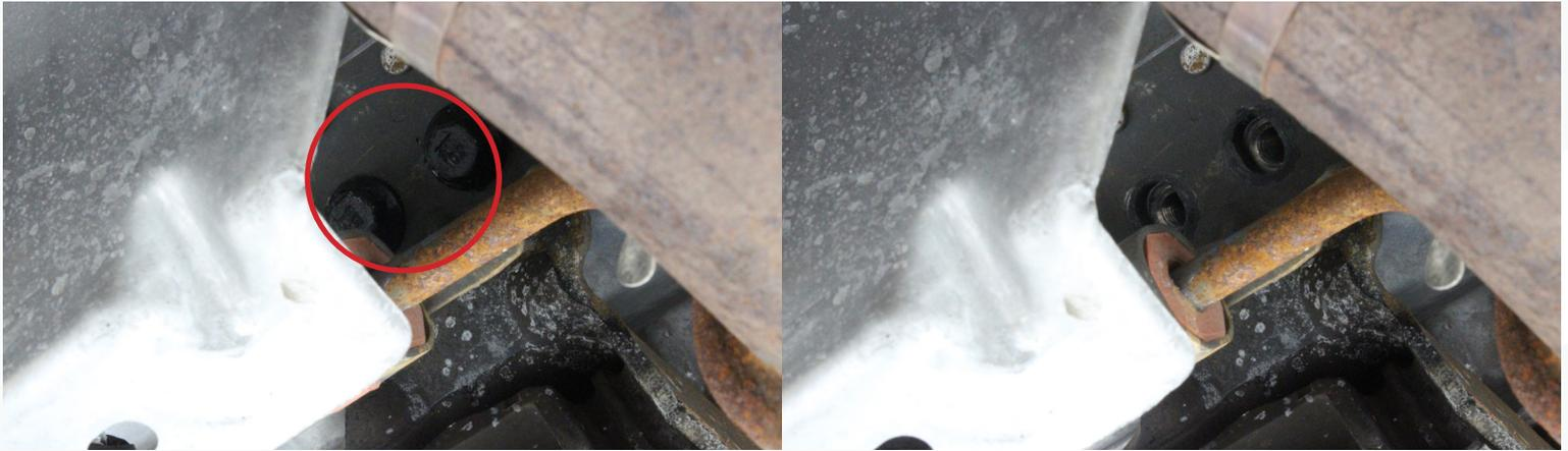
10) Remove the transmission mount from the vehicle.
