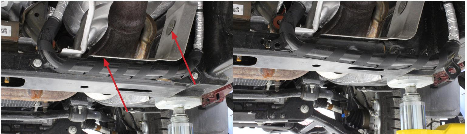
5) Remove the two bolts holding the heat shields on the top of the transmission cross member. There is one and each side of the transmission. These heat shields do not need to be removed, only the bolts
