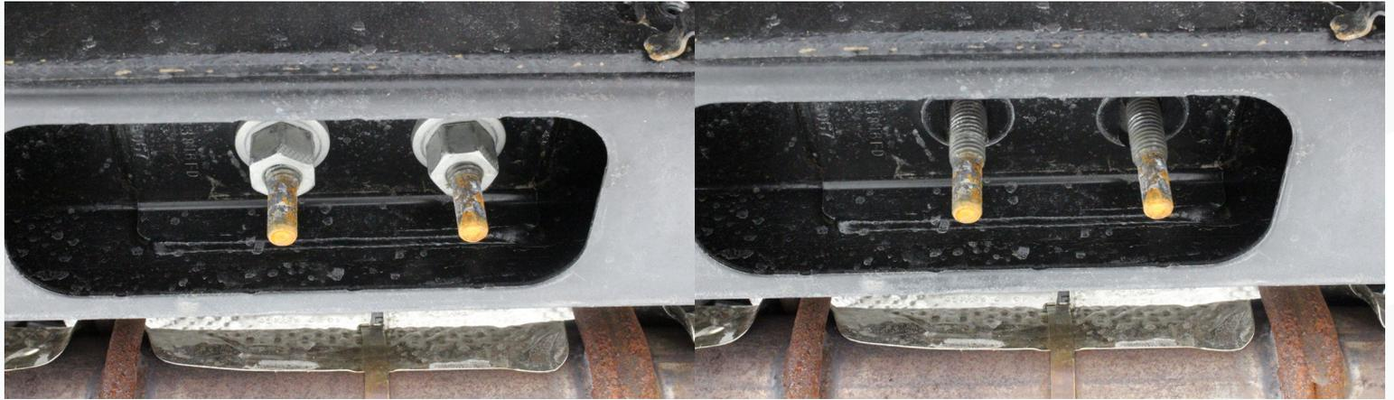
7) Safely support the weight of the transmission and/or transfer case. Remove the two long bolts on each side of the transmissions cross member bolting it to the frame. Remove the transmission cross member from the truck.
