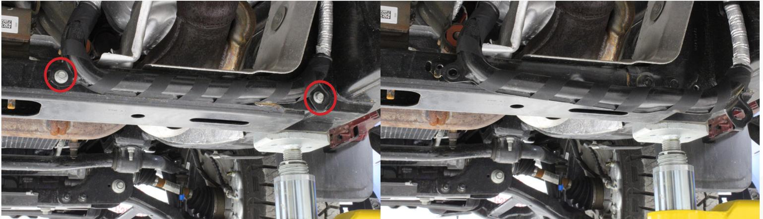
4) Remove the heat shield on the top of the transmission cross member that bolts to the frame.
