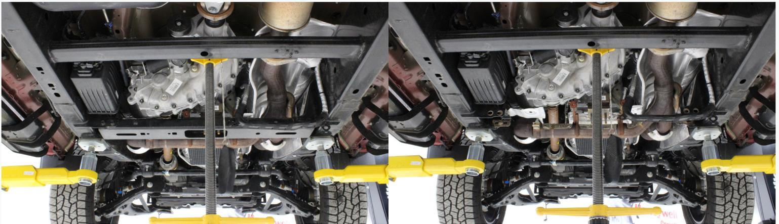
8) Remove the exhaust hanger top clamp and transmission mount bolts on the driver's side
