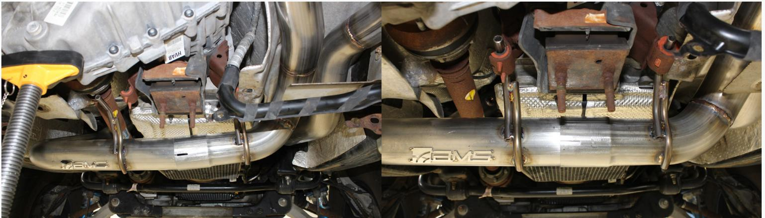
21) Align the butt-joint clamp and the ball flange at the outlet of the downpipes to the catback. The catback will have to be pushed up to align and get the exhaust in the correct position.
