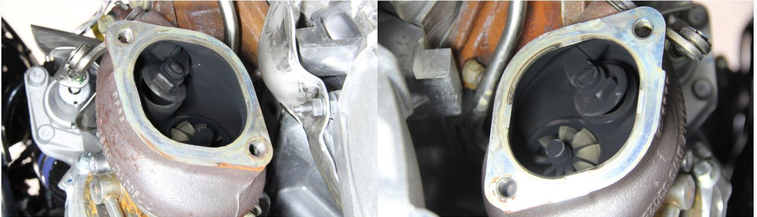
16) Make sure the threads of the turbine housing are clean. Inspect the turbine outlet flange gasket, replace as needed. Install the new AMS turbine outlet flanges using new OEM studs. The best way to do this is to put some washers or spacer on the stud then the nut. Use the nut to tighten the stud in place. Remove the nut by shocking it with an impact to avoid having the stud come out with the nut.
