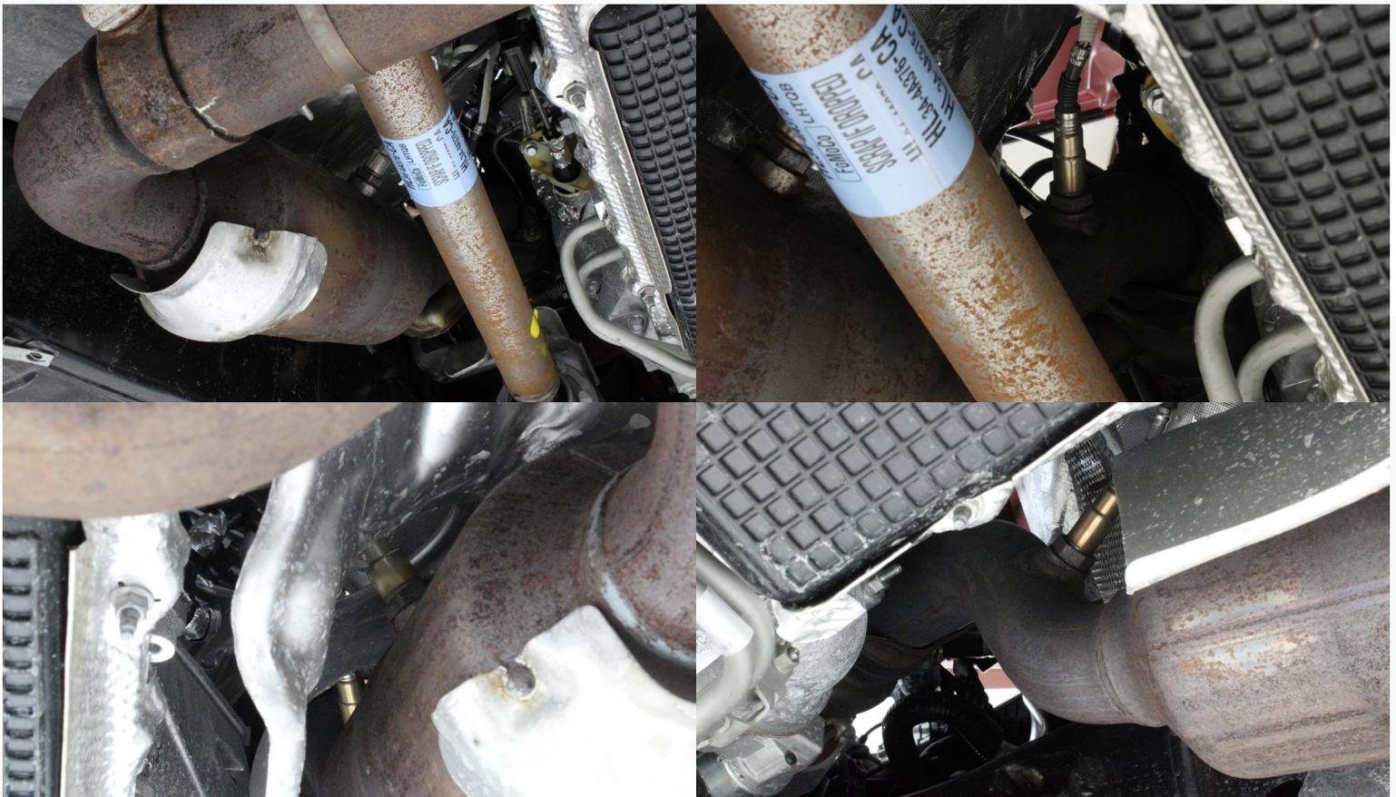
3) On the rear side of the transmission cross member, unbolt and unclip the chassis harness.
