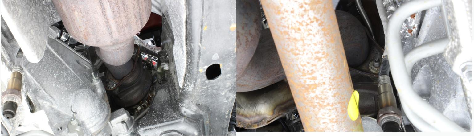
13) Start by removing the passenger downpipe. Once the clamp is off, it is easiest to pull the downpipe up and back, then angle it down and pull it out towards the front of the vehicle. It will take a little back and forth to work it out. The driver side can be removed by taking the front half off the turbine housing, then pulling the rest out. This can be taken out in one piece. Be mindful of the chassis harness that is looped around the downpipes.
