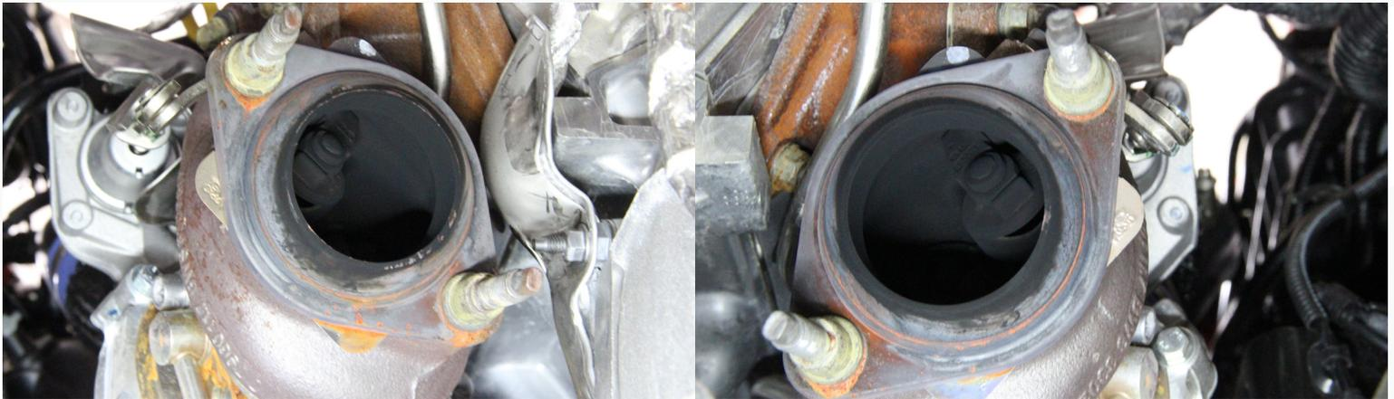
15) Use a 10mm or 3/8" stud extractor to remove the stud from the turbine housing outlet flanges. This may take a little heat on the turbine housing to get these studs to move. Keep in mind to use rust penetrant and do not use an impact. Once you get a stud to unscrew, do so slowly to avoid friction welding the stud in the turbine housing.
