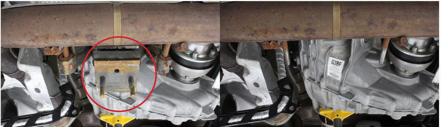
11) Disconnect the two-bolt flange and the butt-joint clamp connecting the downpipe to the rest of the exhaust. Save these bolts they will be reused
