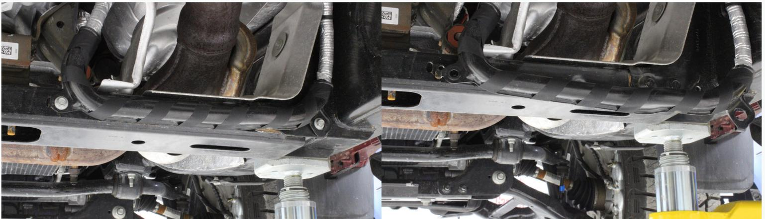
6) Remove the two nuts from the transmission mount.
