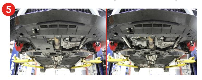
6. Remove both wheel well liners. Remove three 8mm screw, one large push clip, and one large or plastic 10mm nut from under the car. The large 10mm plastic nut is designed to stay in the wheel well liner but may come completely out. Next remove three 10mm plastic nuts and 6 small push clips from inside the wheel well. Remove the wheel well.
