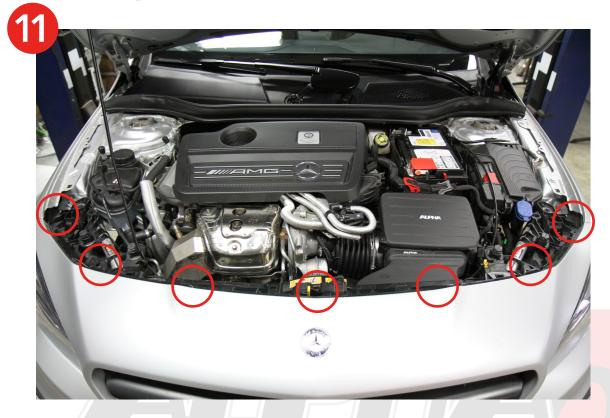
12. A second set of hands to remove the front bumper is highly recommended. Carefully remove the front bumper. Take caution when removing the front bumper so not the scratch the headlights. If your vehicle has any dealer install accessories such as a light up front emblem, there will be a connector you will need to disconnect during removal.
